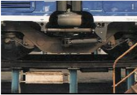
Fig. 2: Traditional metallic bogie for railway rolling stock
