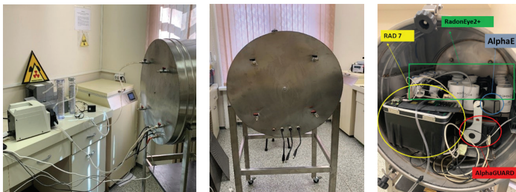
Fig. 3. The ^{222}\text{Rn}/^{220}\text{Rn} laboratory facility at Sofia University (left). Centre: the new 200 L exposure chamber. Right: the exposure chamber filled with radon detectors.
