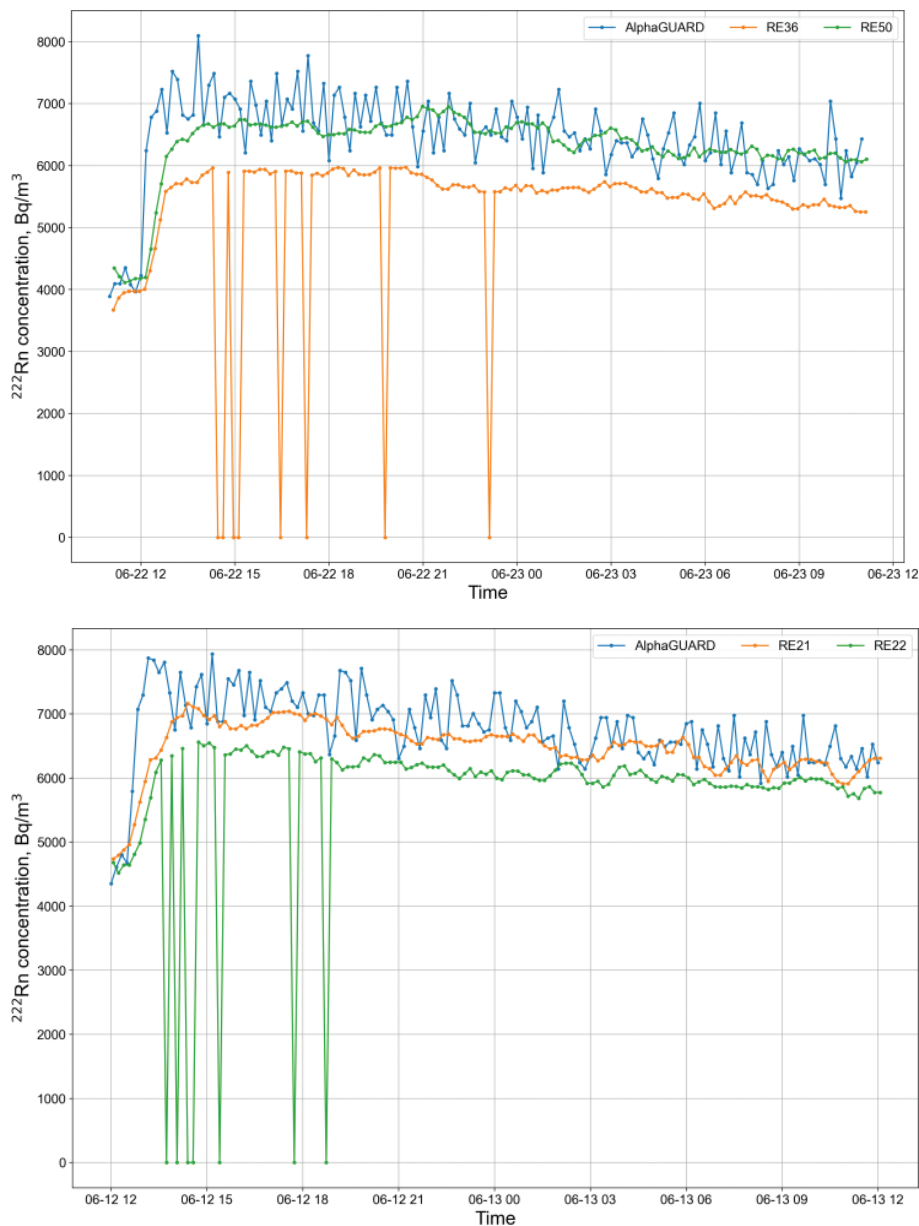
Fig. 7. Examples for saturation of the detectors. When saturated, the detectors record 0 Bq/m 3 – RE36 (orange line) in the left graph and RE50 (green line) in the left graph. The time format on the abscissa is ‘Month-day hour’.
