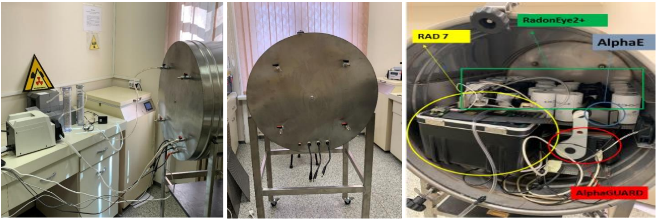
Fig. 3. The ^{222}\text{Rn}/^{220}\text{Rn} laboratory facility at Sofia University (left). Centre: The new 200L exposure chamber. Right: the exposure chamber filled with radon detectors.
