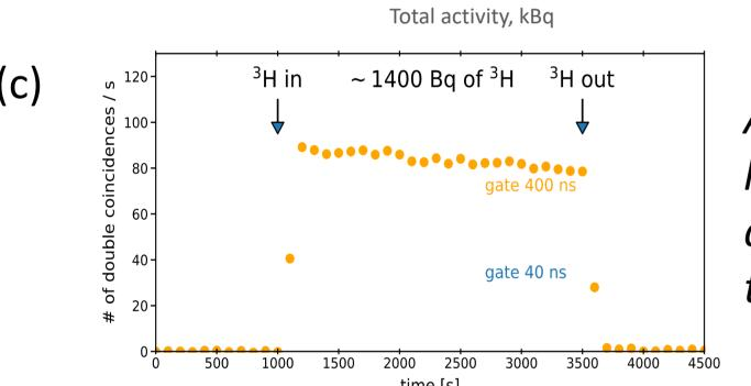
As can be seen on the data to the left, <sup>3</sup>H has been detected at significant counts above the detection limit; comparable to the <sup>85</sup>Kr detections, even if lower.
