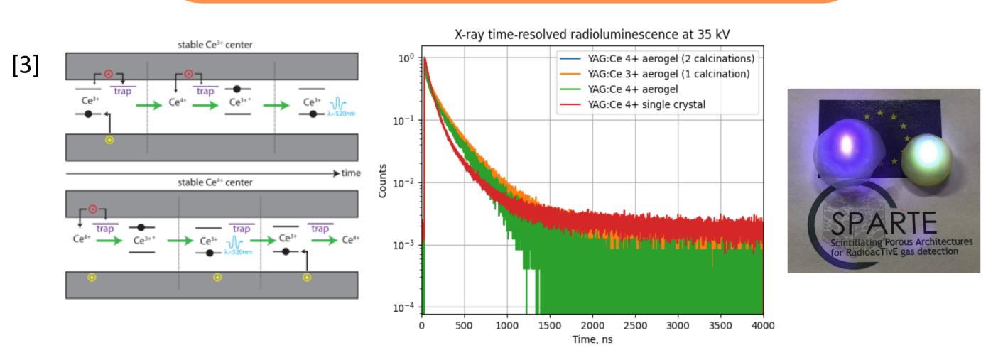
YAG:Ce may contain two species of Ce: Ce<sup>3+</sup> and Ce<sup>4+</sup>. The former is a viable source of photoluminescence, but is a slower emitter during radioluminescence events. The effect is shown to be even more pronounced in materials with many confined spaces such as aerogels.
