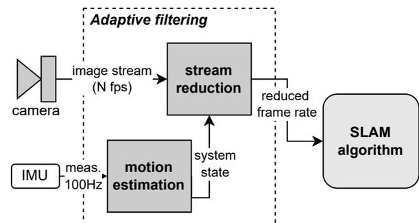
Fig. 1. Functional pipeline for the adaptive filtering approach
