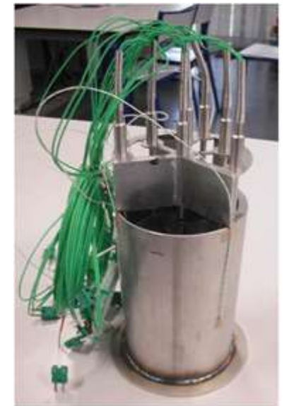
Example of 2L vessel for heating tests of simulated BWPs
