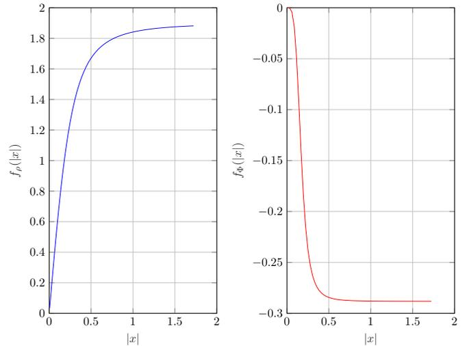
Fig. 5. AM/AM and AM/PM characteristics of Rapp PA [8]
