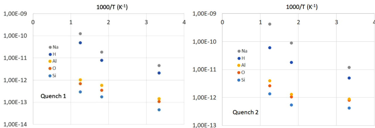
FIGURE 15 Diffusion coefficients (in \text{m}^2 \text{s}^{-1} ) for the five different species in the systems prepared at the thermal quench rates QR1 (left) and QR2 (right)
