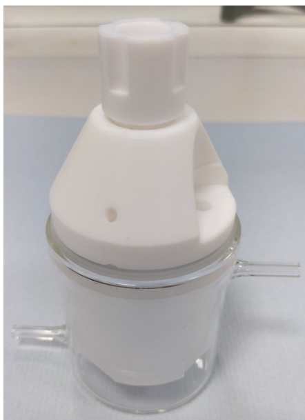
Figure S2. Electrochemical cell designed with Kel-F® and PTFE top.
