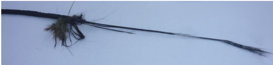
security cable after 2 hours at 750°C
