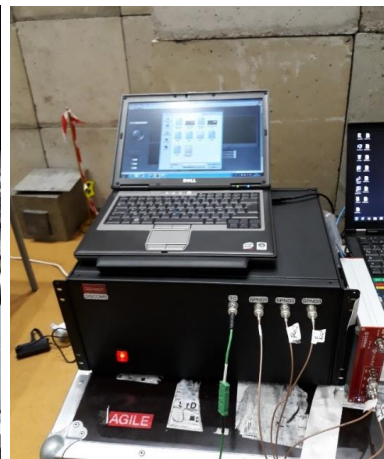
dedicated SPND multi-channel measurement device 375 mA × 24 V power per channel up to 200 m, battery operated
