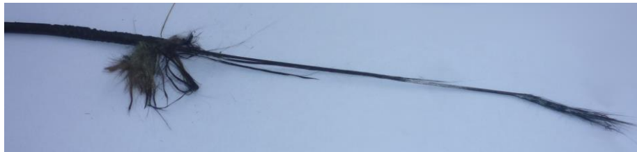
security cable after 2 hours at 750°C
