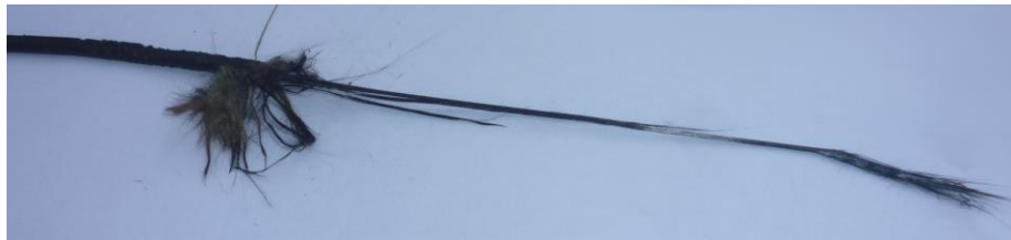
security cable after 2 hours at 750°C
