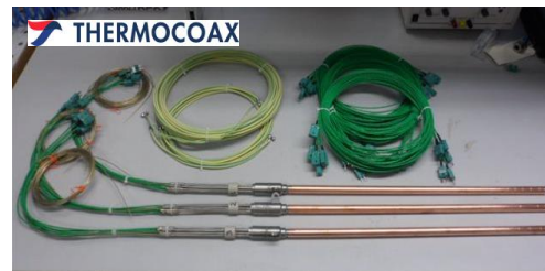
dedicated SPNDs-TC instrumented poles
