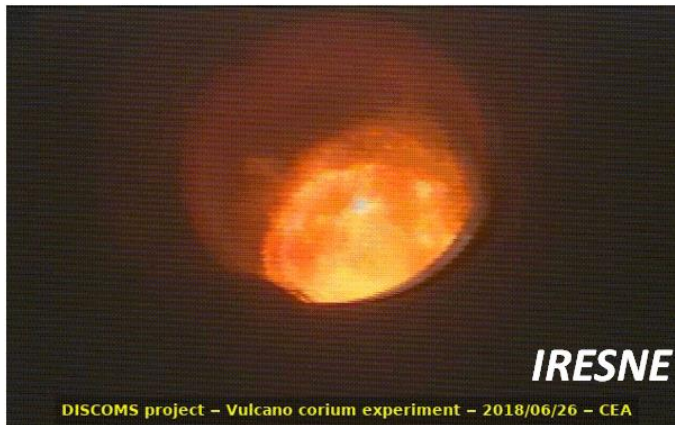
thermite reaction ignition to produce corium
