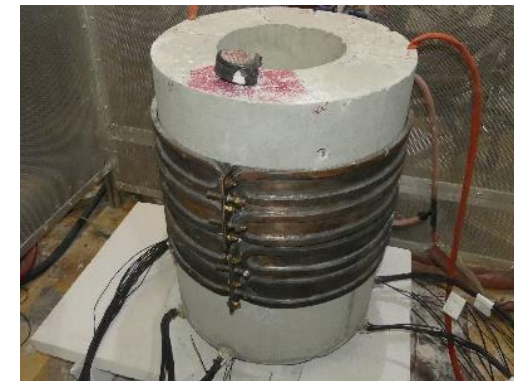
concrete crucible installed with the induction coils at CEA in Cadarache PLINIUS facility
