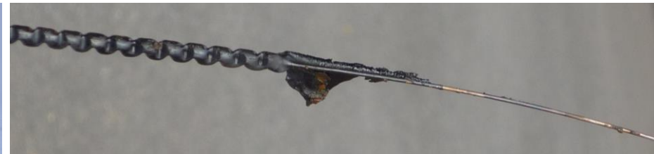
strain sensor cable after heating up to 400°C
