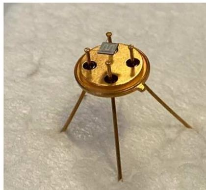
**Figure 6.** *The functional chemical sensor device of ZnO film.*
