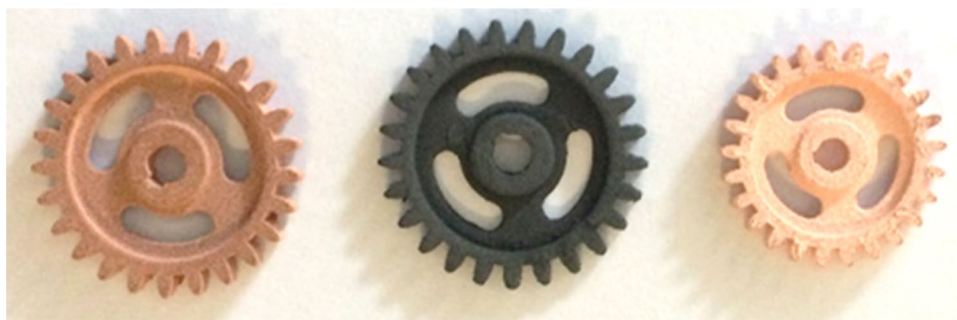
Fig. 12 Gear after DLP process, debinding in air at 400 °C for 4 h (black specimen) and sintering at 1050 °C for 4 h
