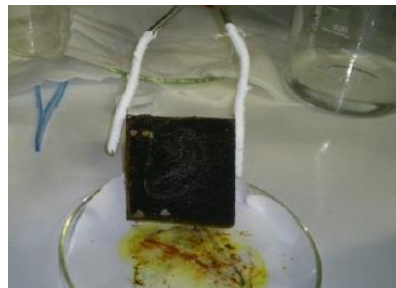
Sample after several etchings ( \approx 100\ \mu\text{m} thickness removed at each etching)
