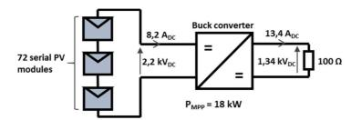
Figure 3 – General schematic of the demonstration PV plant
