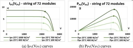
Figure 2 - I<sub>PV</sub>(V<sub>PV</sub>) and P<sub>PV</sub>(V<sub>PV</sub>) characteristics of a 72 PV modules string
