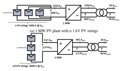
(b) 1 MW PV plant with n/3 3 kV PV strings
