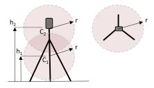
Figure 3: Security volume around each station. Left is front view, right is above view.
