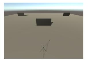
Figure 4: Scene with three walls, 5 m wide and 2.5 m high, placed at 10 m (center) and 30 m (sides) from a LiDAR station.
