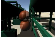
(a) Limited access to platform. Transparent orange spheres are the security volume.
