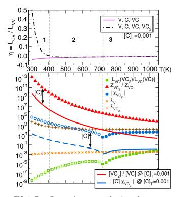
FIG. 1. Top: Drag ratio  $\eta$  as a function of temperature with/without the contribution from  $VC_2$  clusters at  $[C]_T = 10^{-3}$ . Bottom: Various ratios of cluster quantities as a function of temperature. The ones in the bottom legend depend on  $[C]_T$  while the ones in the top legend are combinations of intrinsic cluster properties. All curves are independent of  $[V]_T$ . Open symbols and dashed lines represent negative quantities.
