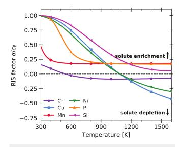
**FIG. 1.** RIS factor for various solutes in  $\alpha$ -Fe, which provide the RIS tendency at PD sinks (solute enrichment or depletion).<sup>42</sup>  $c_{\rm B}$  is the solute concentration ( $X_{\rm B}$  in our notations). Reproduced with permission from Messina *et al.*, Acta Mater. **191**, 166 (2020). Copyright 2020 Elsevier.
