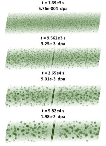
**FIG. 6.** AKMC simulations of  $\alpha$ - $\alpha'$  phase separation in Fe-15 at. % Cr under an irradiation at 290 °C and  $3.4 \times 10^{-7}$  dpa s<sup>-1</sup>, with a negative segregation energy of Cr on the GB and on the neighboring planes, leading to the equilibrium segregation of Cr on the GB.<sup>113</sup> Reproduced with permission from Soisson and Jourdan, Acta Mater. **103**, 870 (2016). Copyright 2016 Elsevier.
