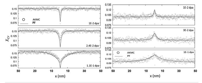
**FIG. 4.** RIS profiles obtained using AKMC (symbols) and PF (lines) in Fe–15 at. %Cr at 900 K (left) and in Fe–10 at. %Cr at 700 K (right), as a function of the distance from the GB, x, and for different irradiation doses at a dose rate of  $10^{-5}$  dpa s<sup>-1</sup>.<sup>103</sup> Reproduced with permission from Piochaud *et al.*, Comput. Mater. Sci. **122**, 249 (2016). Copyright 2016 Elsevier.
