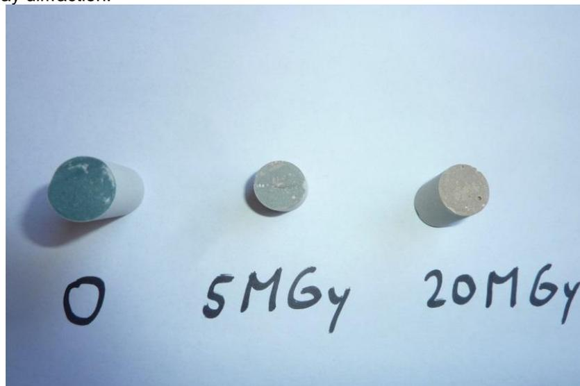
Figure 3. Splits of cement pastes P-4 (1 cm by diameter) containing NaNO<sub>3</sub> after gamma irradiation (5 and 20 MGy) and reference pastes (non irradiated).
