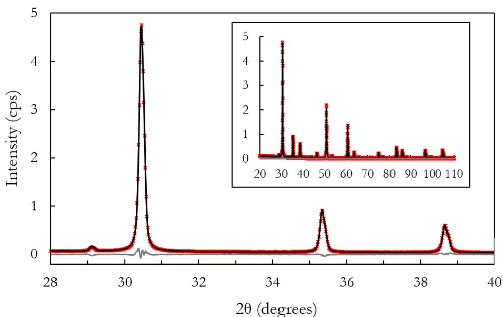
Figure 2: Zoom showing the comparison between the experimental (red cross) and refined (black line) diffraction pattern with associated errors (grey line) collected on sample annealed 600 minutes at 1050°C. The inset displays the full diagram with the refinement and associated errors. The quality of the refinement is justified by the very good agreement between the measured and computed patterns. (2-column fitting figure, color should be used)
