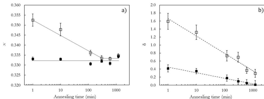
Figure 6: Evolution of the reduced atomic position  $x$  (a) and oxygen sub-stoichiometry  $\delta$  (b) in  $Y_2Ti_2O_{7-\delta}$  powders annealed under oxygen flow at 900°C (open symbols) and 1050°C (black symbols). (2-column fitting image)
