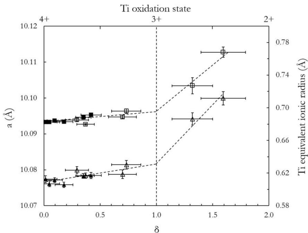
Figure 7: Increasing of lattice parameter  $a$  (squares) and  $Ti$  ionic radius (triangles) with oxygen sub-stoichiometry ( $\delta$ ), due to  $Ti$  oxidation state variations in  $Y_2Ti_2O_{7-\delta}$  powders annealed at 900°C (open symbols) and 1050°C (black symbols). (1-column fitting figure)
