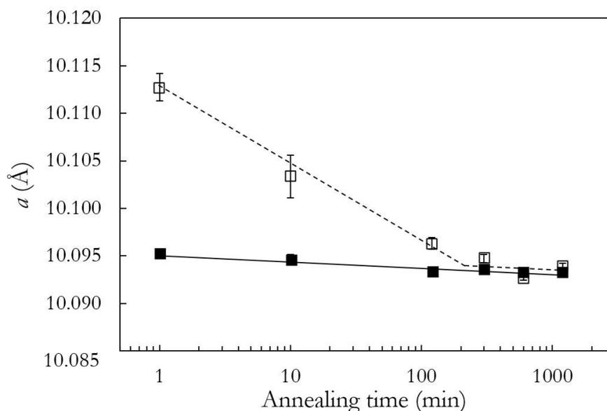
Figure 5: Evolution of the unit lattice parameter with annealing time at 900°C (open squares and dashes) and 1050°C (black squares and full line). Errors bars associated with the evolution of  $a$  are also plotted. (1-column fitting figure)
