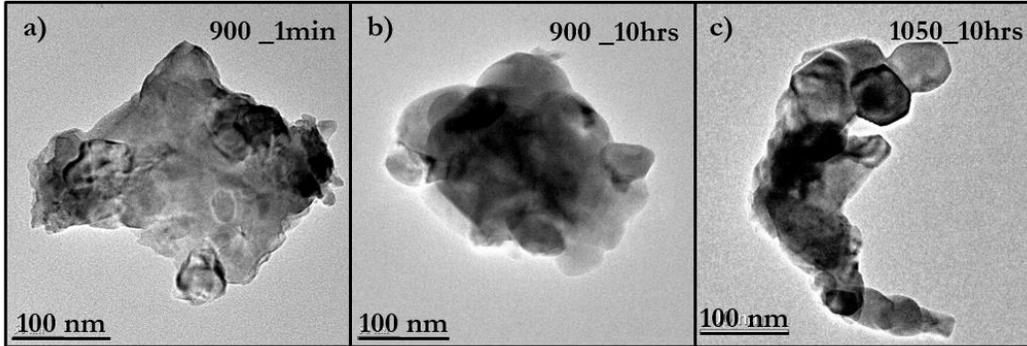
Figure 3: TEM micrographs of 900\_1, 900\_600 and 1050\_600 annealed particles. Increasing the annealing time, grains become spherical. (2-column fitting figure)
