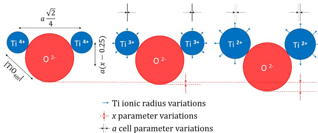
Figure 8: Schematic description of the variations of the reduced atomic position  $x$ , unit cell parameter  $a$  and Ti–O distance induced by changing Ti oxidation state in a sub-stoichiometric pyrochlore structure. Atoms are roughly on scale. (2-column fitting figure, color to be used)
