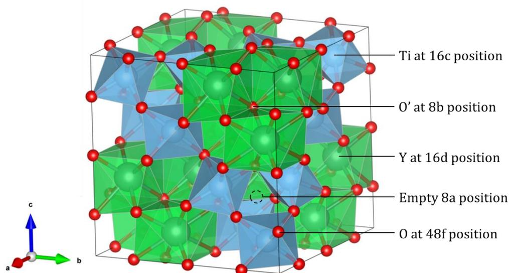
Figure 1:  $Y_2Ti_2O_7$  ideal pyrochlore structure. Green distorted cubes and blue distorted octahedra correspond to Y and Ti cations coordination environments, respectively. (2-column fitting figure, color should be used)
