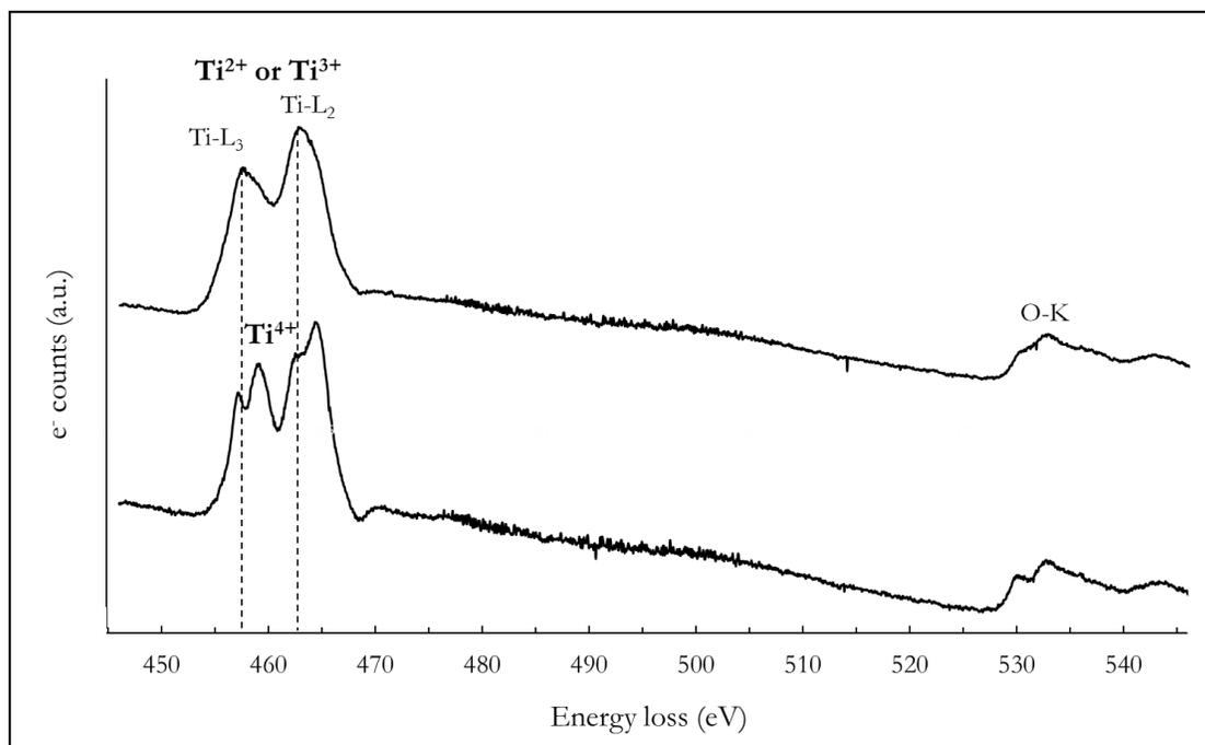
Figure 9: Background-subtracted EELS spectra focused on  $Ti-L_{2,3}$  and  $O-K$  edges acquired in the same conditions on two different aggregates of 900\_1  $Y_2Ti_2O_{7-\delta}$  pyrochlore powder. Reduced  $Ti$  (up) and  $Ti^{4+}$  (bottom) cations are identified. (2-column fitting figure)
