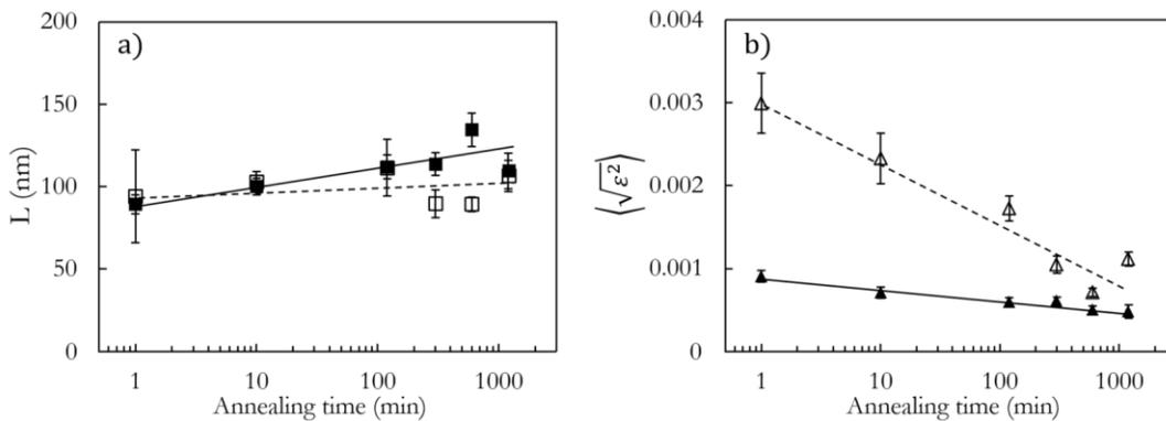
Figure 4: Evolution of CDD (a) and micro-strains (b) extracted from the HW analysis with annealing time. Powders annealed at 900°C (open symbols and dashes) exhibit larger variations in micro-strains than those treated at 1050°C (black symbols and full line). Only slight coarsening is observed with time for both of the annealing temperature. (2-column fitting figure)
