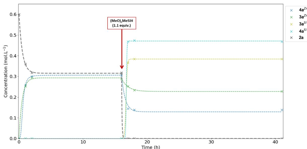
Figure 1. Time-step analysis by <sup>1</sup>H NMR spectroscopy of the stepwise stoichiometric reduction of **2a** by complex **1** and DMMS.
