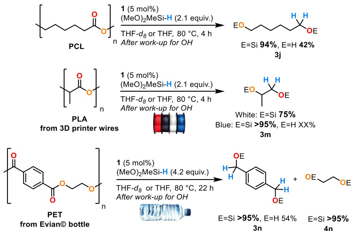
Scheme 5. Reductive depolymerisation of polyesters catalysed by complex **1**. The yields of silyl ethers were measured by  $^1\text{H}$  NMR spectroscopy by integration against mesitylene as an internal standard (reactions conducted in  $\text{THF-}d_8$ ). The yields of alcohols are isolated yields from reactions in THF after basic workup.
