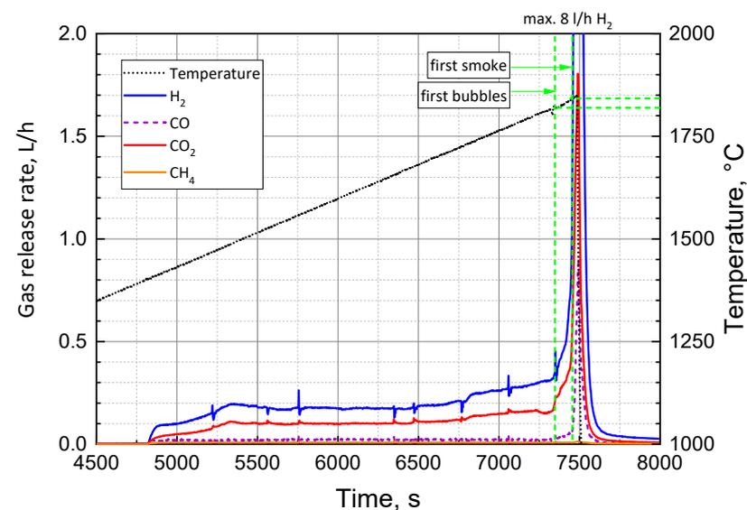
**Figure 3.** Temperature history and gas release rates during transient test SiC-01.
