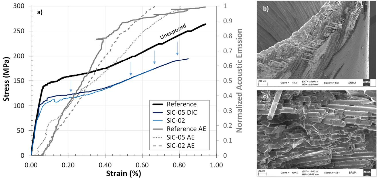
**Figure 11.** (a) Uniaxial tensile stress-strain behavior measured on SiC-02 and SiC-05 samples at ambient temperature after 1 h isothermal oxidation in steam at 1700 °C. The reference stress-strain curve measured on the pristine material is given for comparison. (b,c) Representative fracture surface SEM images observed at different magnitudes on sample SiC-02.
