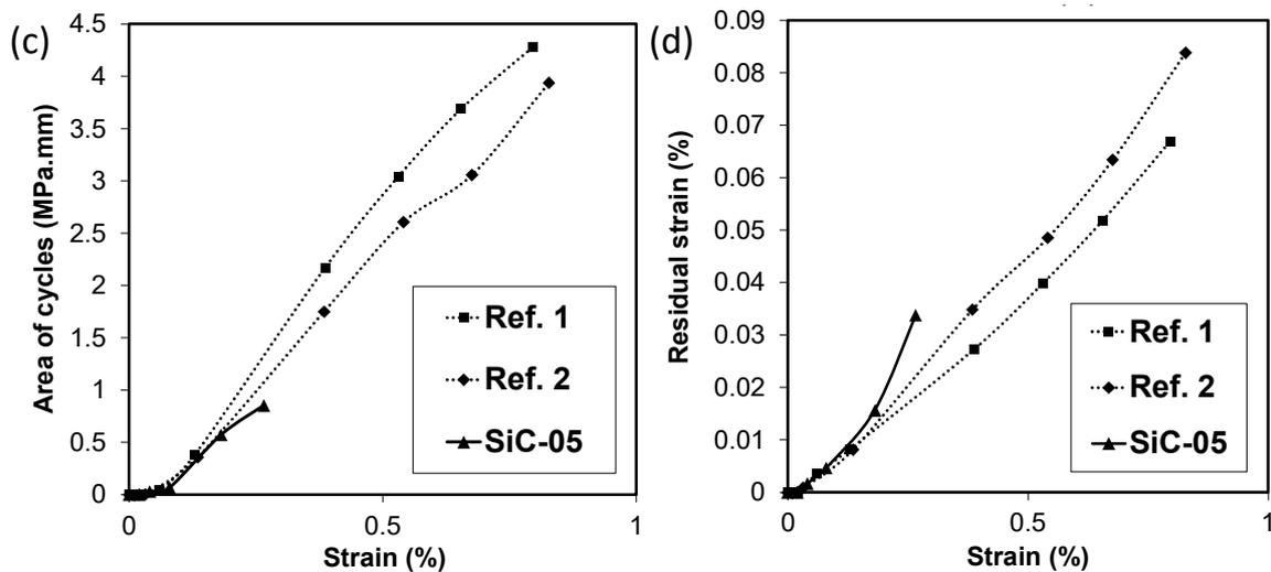
**Figure 13.** Reduced modulus (a), Full width at half-maximum (b), Area of the cycles (c), and Residual strains after unloading (d) as a function of the strain before unloading for reference materials (Ref. 1 and Ref. 2) and SiC-05.
