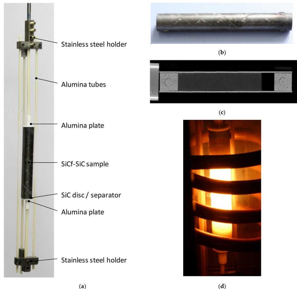
**Figure 2.** QUENCH-SR facility and  $\text{SiC}_f\text{-SiC}$  sample. (a) Sample holder; (b)  $\text{SiC}_f/\text{SiC}$  sample before test; (c)  $\text{SiC}_f\text{-SiC}$  sample before test (tomography); (d) Sample in QUENCH-SR rig at 1700 °C.
