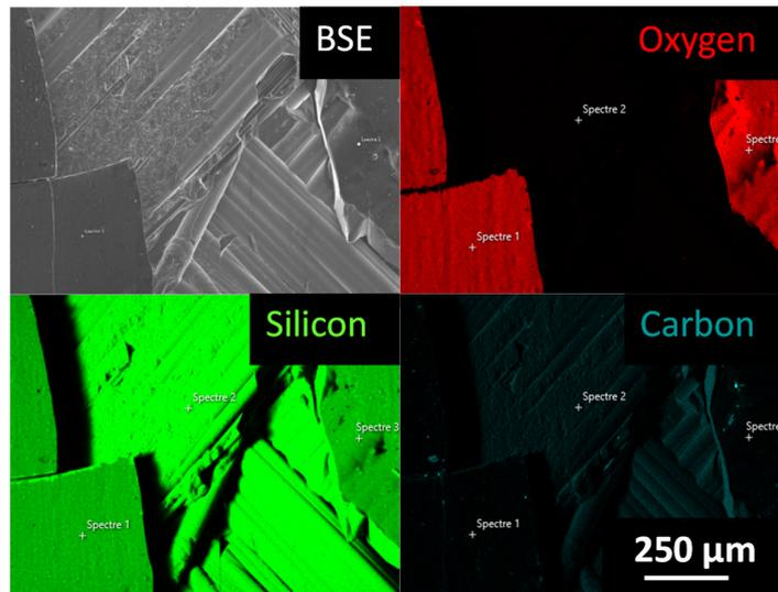
**Figure 12.** BSE and oxygen, silicon and carbon element mappings (EDS) of the SiC-02 surface after mechanical test up to failure. No oxygen content is measured under the sealcoat, which was removed during the tensile test.
