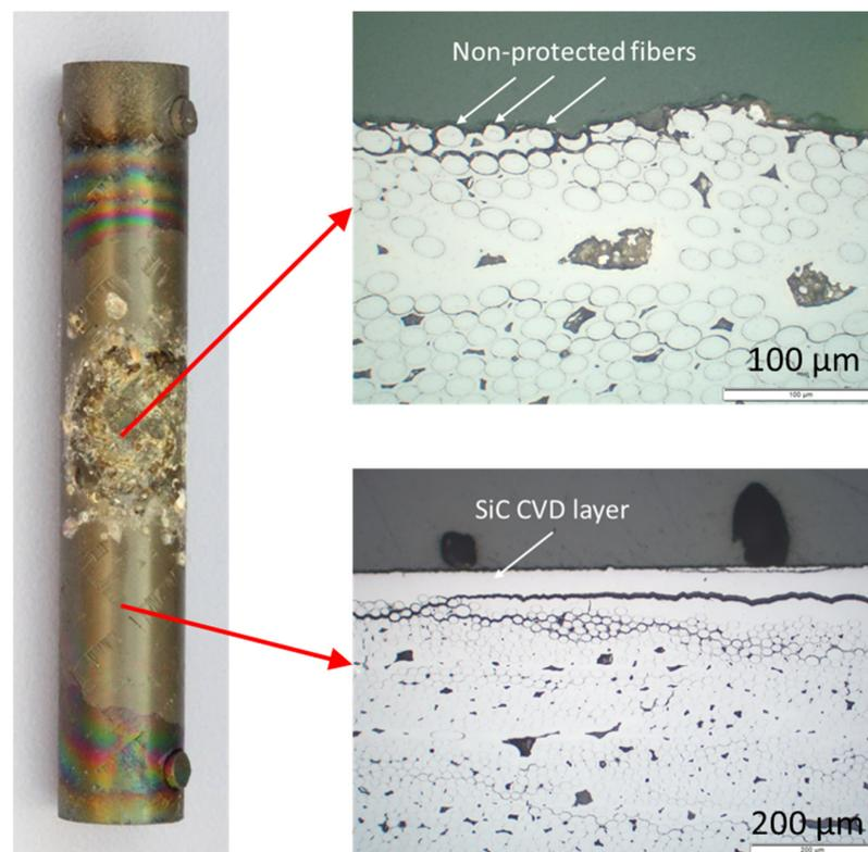
**Figure 5.** Post-test appearance of the sample after the transient test up to 1845 °C and optical micrographs from the failure region in the middle of the sample and from the non-failure region below.
