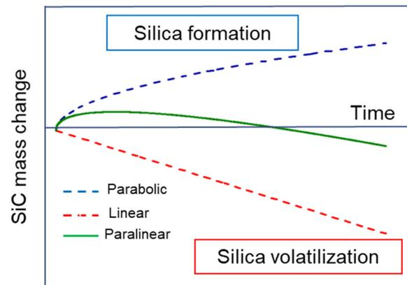
**Figure 1.** Paralinear mass change during HT oxidation of SiC due to formation and volatilization of a superficial SiO<sub>2</sub> scale.
