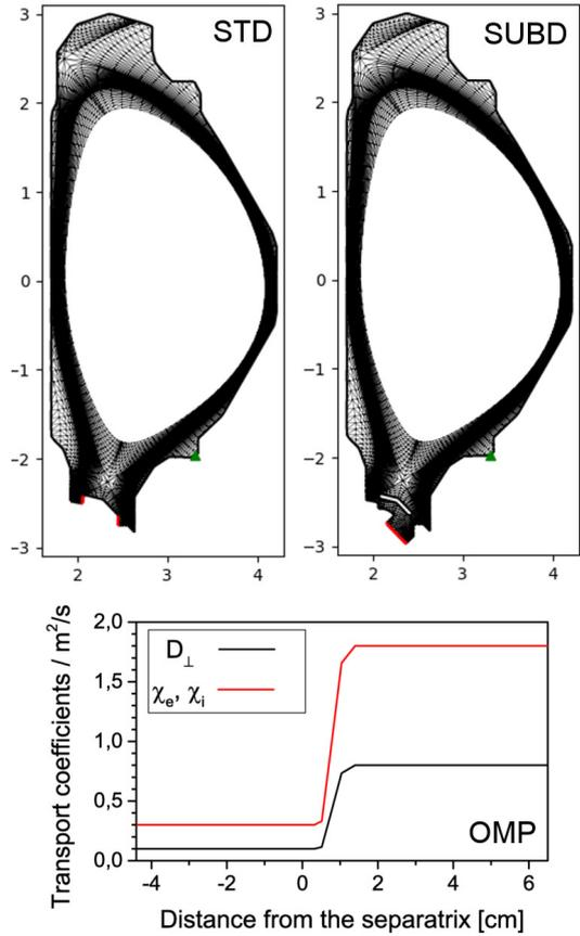
Figure 1: The meshes used: (STD) with two pumping surfaces, (SUBD) with subdivertor structure and one pumping surface. The position of pumps is marked by red line. D fuelling valve position is marked by  $\blacktriangle$ . Outer midplane profiles of particle radial diffusion coefficient  $D_{\perp}$  and electron and ion heat radial conductivities  $\chi_e$ ,  $\chi_i$ , respectively, are presented below (OMP).
