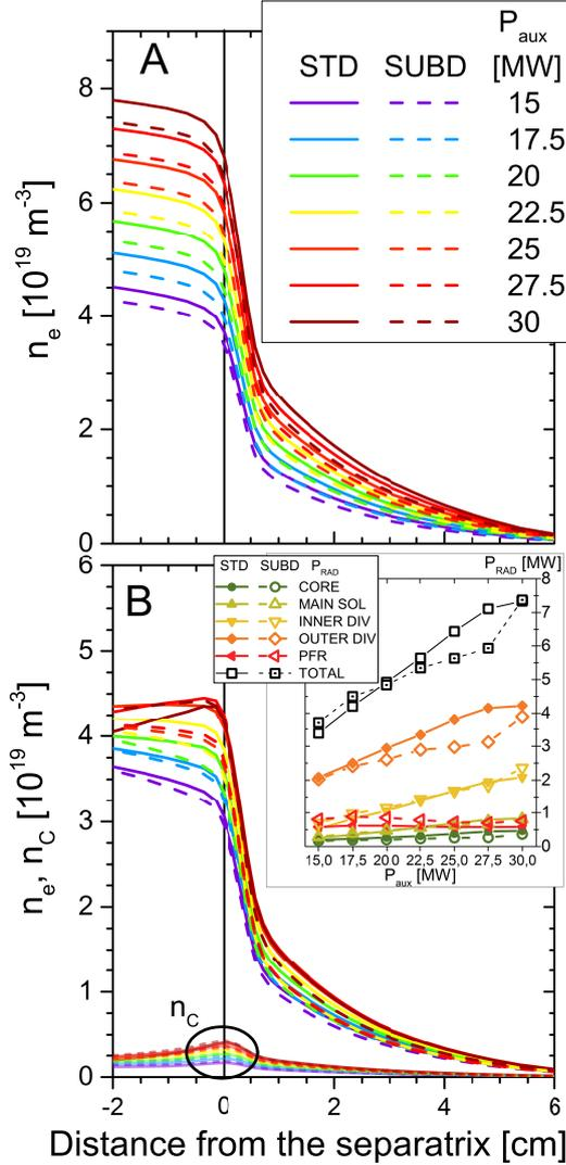
Figure 3: The OMP  $n_e$  profiles for both geometries in  $P_{\text{aux}}$  scan: (A) presents the results for pure D plasma and (B) with C impurity. In this case also total C concentration profile is presented. The inset: C radiation power split into regions: CORE - confined plasma, MAIN SOL - main chamber SOL, INNER DIV/OUTER DIV - inner/outer divertor volume, PFR - private flux region.
