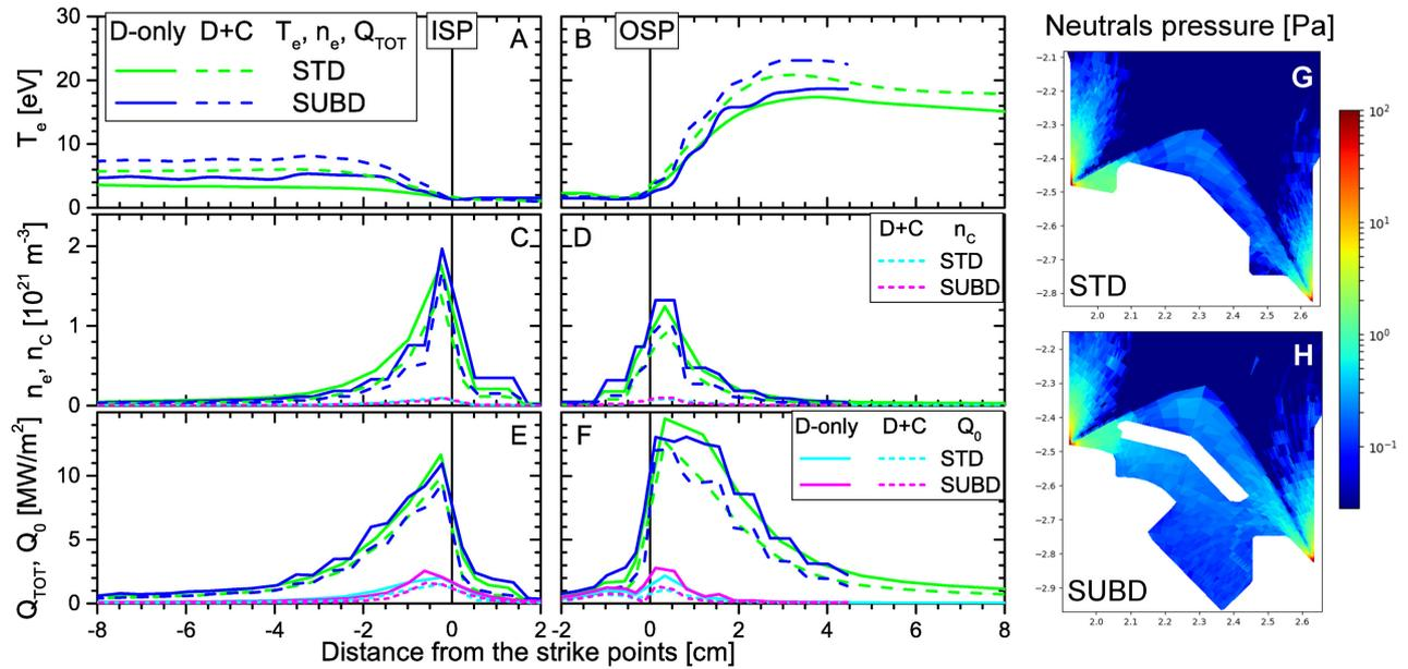
Figure 4: Comparison of the inner and outer target profiles for the  $P_{aux}=15$  MW case: (A, B) - electron temperature, (C, D) - electron density and carbon density, (E, F) - total heat load  $Q_{TOT}$  and the contribution of neutral particles  $Q_0$ . ISP and OSP - inner and outer strike point, respectively. (G, H) - the neutral pressure in the divertor and subdivertor volume for the cases with C.
