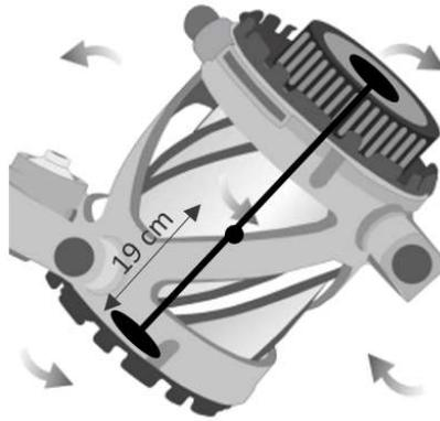
Figure 2: Schematic of the Turbula motion wherein powders are subjected to periodic translational and rotational movements to achieve blending (Schematic source: <https://aerosol-soc.com/wp-content/uploads/2016/06/1500-Hertel-Pent-Thurs-v1.pdf>).
