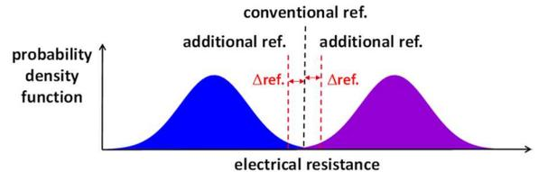
Fig. 7: Weak-bit-identification based on sensing with additional reference values. The logarithm of the electrical resistance may be considered on the X-axis for log-normal distributions of the electrical resistance states.
