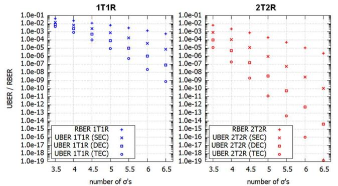
Fig. 4: RBER and UBERs vs.  $\sigma$ -distance (number of  $\sigma$ 's) between LRS and HRS for 32-bit 1T1R and 2T2R memories. The  $\sigma$ -distance between LRS and HRS is defined according to annex I.
