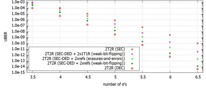
Fig. 10: UBER vs.  $\sigma$ -distance between LRS and HRS for a 32-bit 2T2R memory protected by a SEC-DED code with weak bits identified as illustrated in Fig. 6 and Fig. 7.
