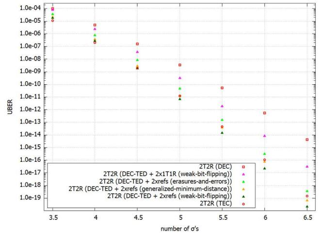
Fig. 12: UBER vs.  $\sigma$ -distance between LRS and HRS for a 32-bit 2T2R memory protected by a DEC-TED code with weak bits identified as illustrated in Fig. 6 and Fig. 7.
