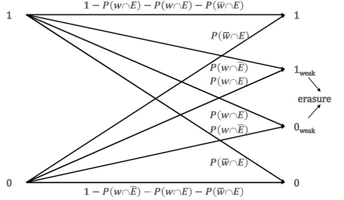
Fig. 5: Equivalent channel model with transition probabilities between programmed and sensed values.  $E$  and  $w$  represent events associated to an erroneous bit or an identified weak bit in a sensed memory word, respectively. An overline indicates a complementary event. The symbol ' $\cap$ ' stands for event intersection.
