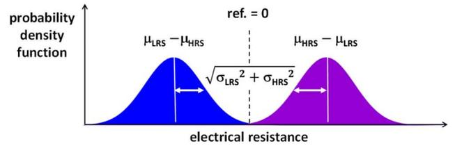
Fig. 3: Distribution of the differences between HRS and LRS used to encode logical values in a 2T2R cell configuration.
