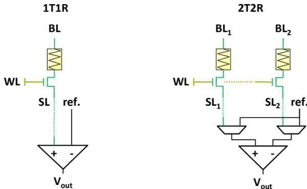
Fig. 1: 1T1R and 2T2R cell configurations with connections to word line (WL), bit lines (BL), source lines (SL) and sense amplifier. In 2T2R cell configurations, a *ref* value is used to verify in 1T1R mode the separation between the LRS and HRS values programed during memory write operations.
