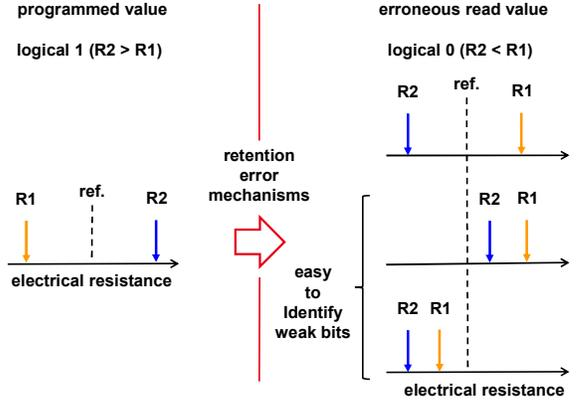
Fig. 6: Retention error mechanisms in a 2T2R cell configuration.
