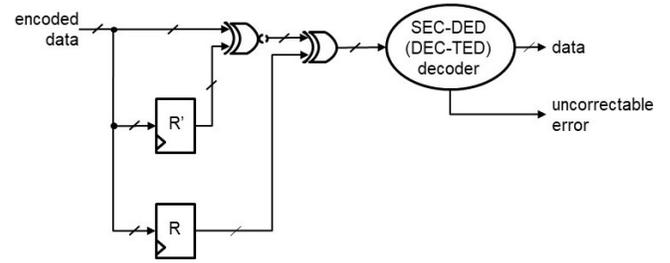
Fig. 13: Glue logic that may be used to implement weak-bit-flipping in front of a conventional errors-only decoder.
