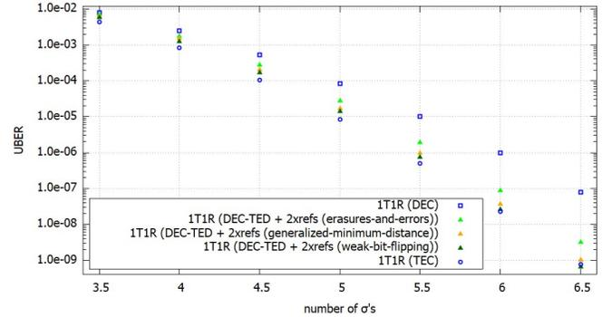
Fig. 11: UBER vs.  $\sigma$ -distance between LRS and HRS for a 32-bit 1T1R memory protected by a DEC-TED code with weak bits identified as shown in Fig. 7.
