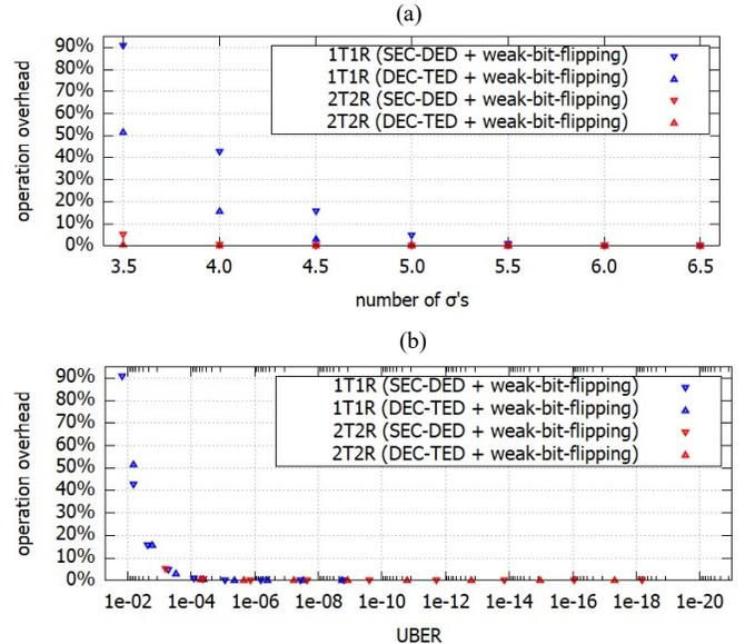
Fig. 14: Memory sense and ECC decode overhead vs. (a)  $\sigma$ -distance between LRS and HRS and (b) achieved UBER.
