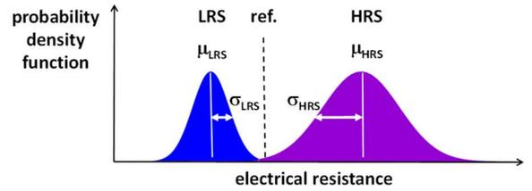
Fig. 2: Distribution of the electrical resistances in low resistance states (LRS) and high resistance states (HRS) for a 1T1R cell configuration with 1 bit per cell.
