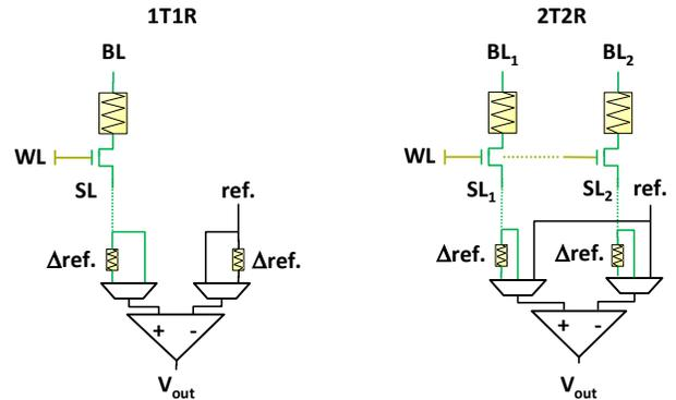
Fig. 8: Possible implementation of sensing with additional reference values as illustrated in Fig. 7.
