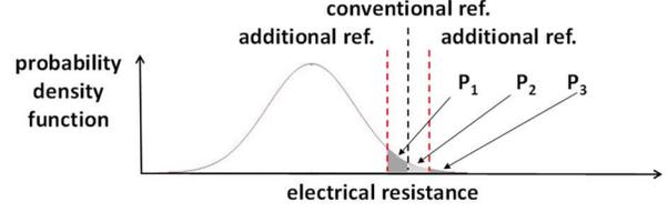
Fig. 15: Graphical representation of the probabilities  $P_1$ ,  $P_2$ ,  $P_3$  for the left-hand side distribution in Fig. 7.
