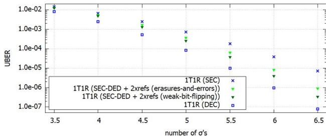
Fig. 9: UBER vs.  $\sigma$ -distance between LRS and HRS for a 32-bit 1T1R memory protected by a SEC-DED code with weak bits identified as shown in Fig. 7.
