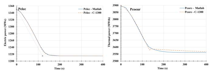
Fig. 8. Electrical and thermal power for the Matlab load-following validation case.
