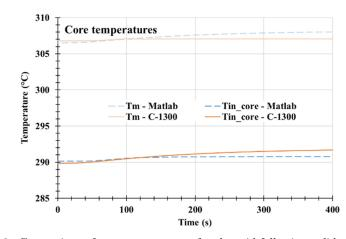
Fig. 10. Comparison of core temperatures for the grid-following validation case.
