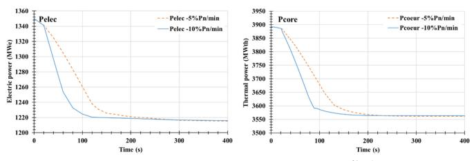
Fig. 11. Electrical and thermal power for a constrained transient at -10%Pn/min.
