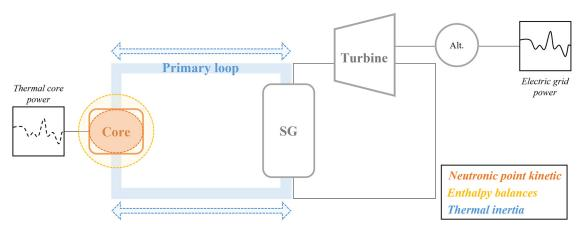
Fig. 6. Diagram of the simplified modelling of a 1300 MW PWR type reactor.
