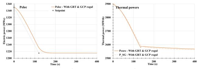
Fig. 3. Electrical and thermal powers (core Pcore and steam generator P\_SG) during a load following transient.
