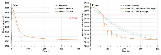
Fig. 9. Comparison of electrical and thermal power for the grid-following validation case.
