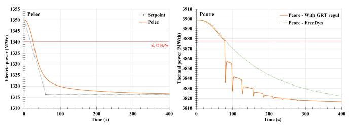
Fig. 1. Electrical and thermal powers during a primary frequency control transient.
