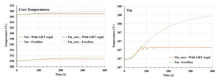
Fig. 2. Temperatures in the core including the average temperature in the core  $(T_m)$  and inlet core temperature  $(Tin\_core)$  during a primary frequency control transient.
