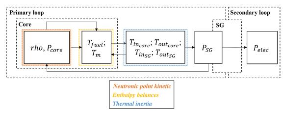
Fig. 7. Schematic of the quantities for the global modelling of the reactor.
