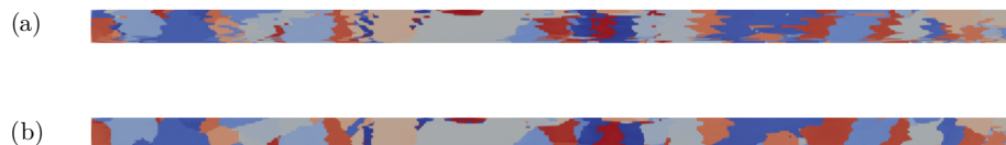
Figure 20. Stacking of successive 2D EBSD maps to reconstruct the 3D microstructure, (a) without and (b) with the use of Eq. 15
