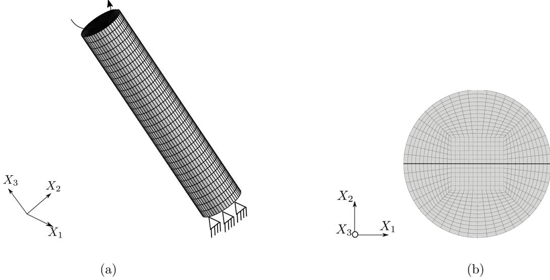
Fig. 4: Microwire torsion (a) boundary conditions (b) example mesh from the top side in which the black line represents an initial material line. For the  $\langle 001 \rangle$  crystal orientation the black line is oriented along a  $\langle 110 \rangle$  direction. For the  $\langle 111 \rangle$  crystal orientation it is oriented along a  $\langle 11\bar{2} \rangle$  direction.
