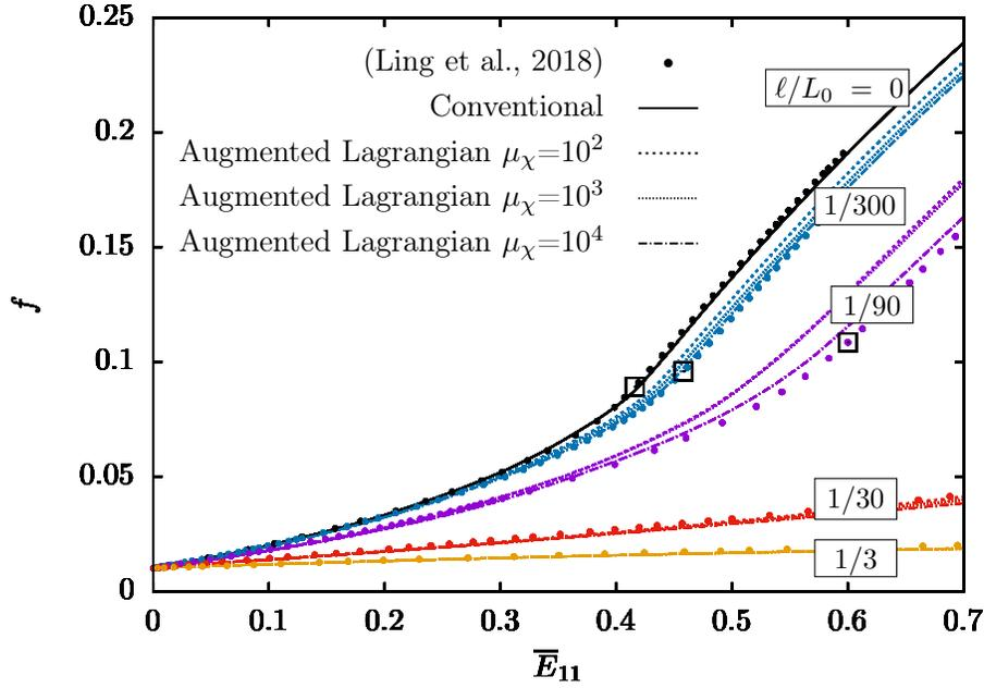
Fig. 14: Void volume fraction  $f$  evolution with respect to macroscopic deformation  $\bar{E}_{11}$  for different intrinsic length to cell size ratios  $\ell/L_0$  obtained with the micromorphic (solid lines) and the augmented Lagrangian (dashed lines) formulations in porous unit-cell simulations with  $f_0 = 0.01$  and material parameters presented in Table 5. Hollow squares denote onsets of void coalescence.
