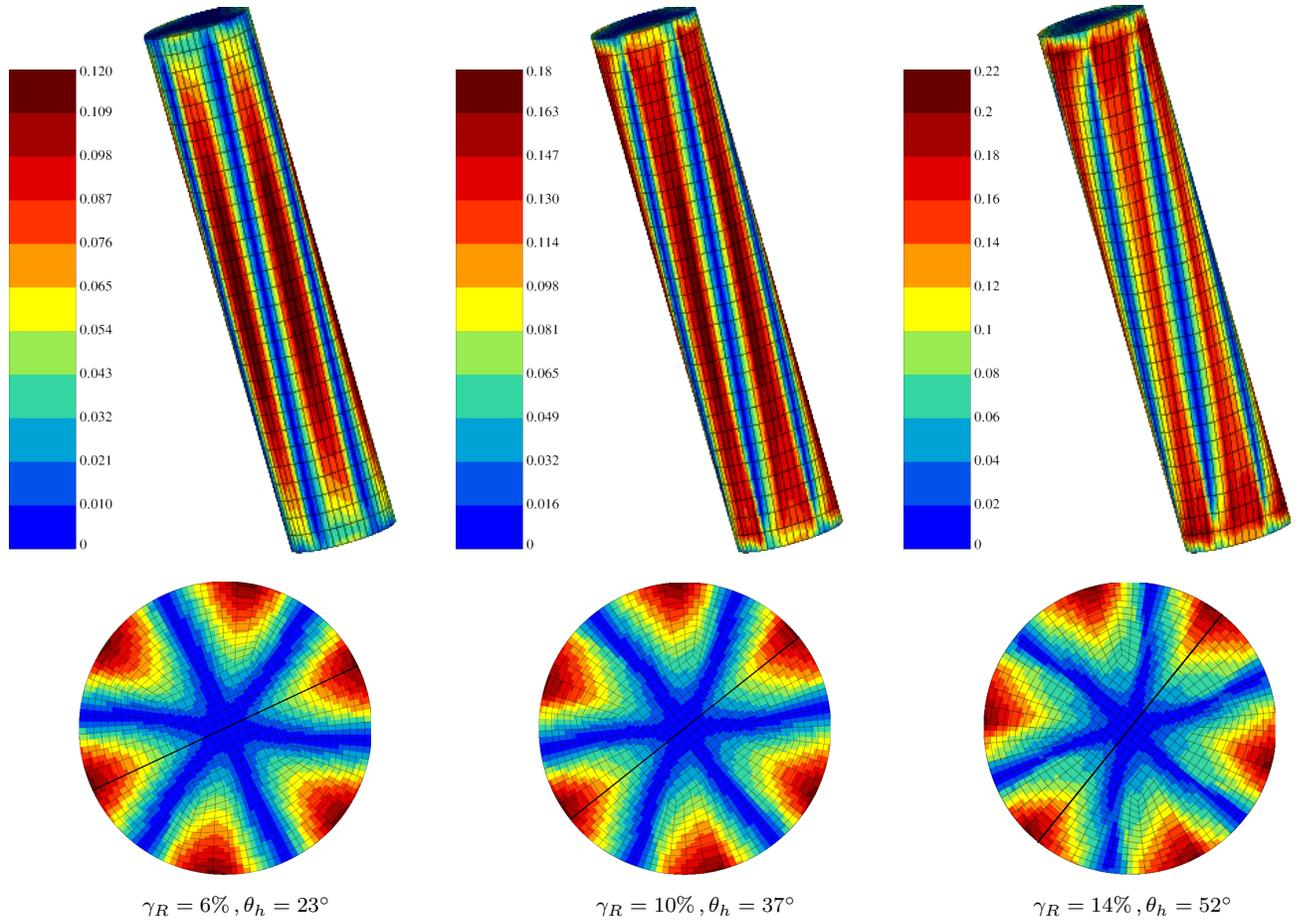
Fig. 6: Cumulative plastic strain ( $\gamma_{cum}$ ) field in FCC single crystal for  $\langle 111 \rangle$  crystal orientation in classical crystal plasticity with respect to deformed configuration. The material line shown in Fig. 4b and its rotation with increasing surface strain are shown by a black line on the cross-section.
