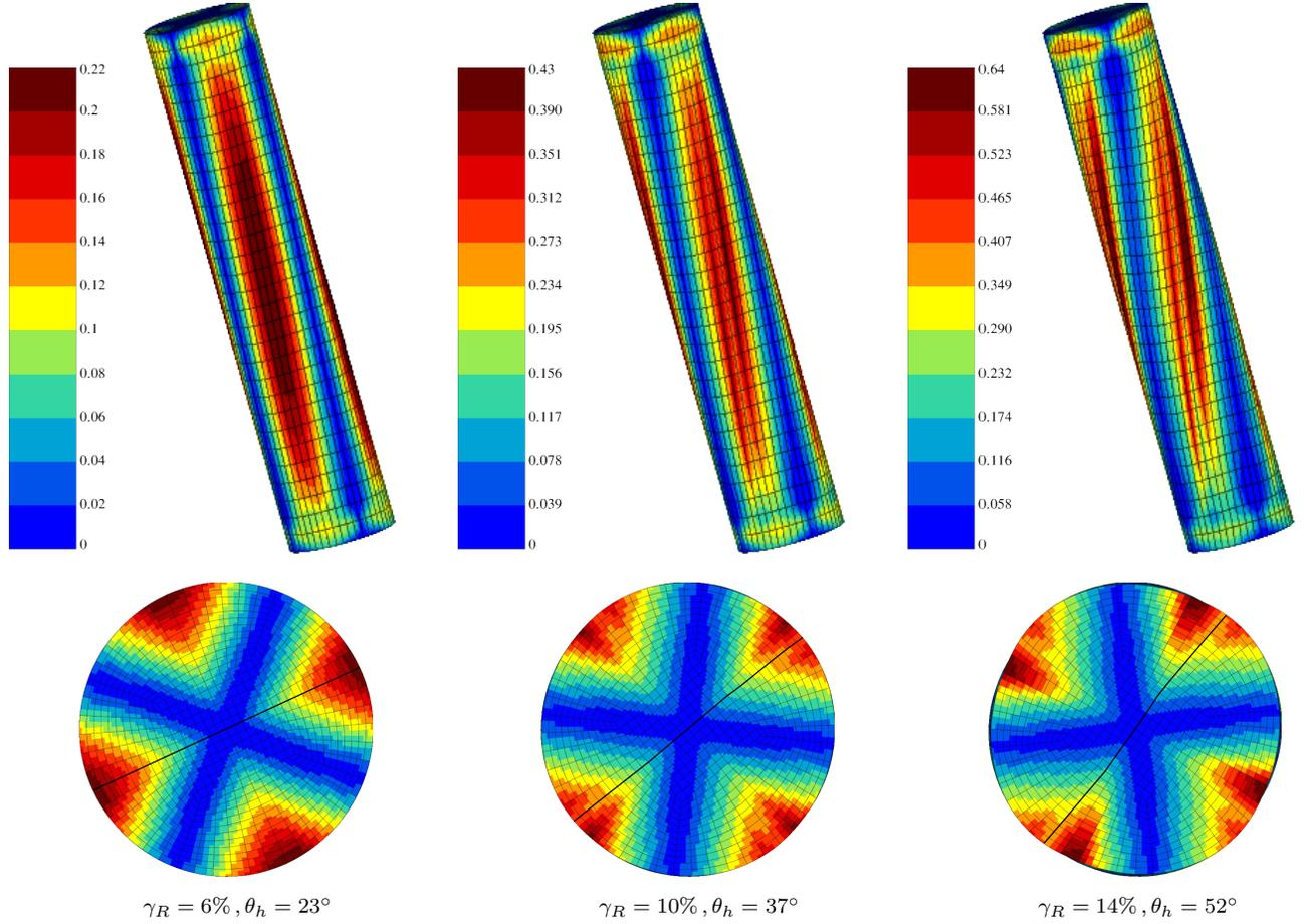
Fig. 5: Cumulative plastic strain ( $\gamma_{cum}$ ) field in FCC single crystal for  $\langle 001 \rangle$  crystal orientation in classical crystal plasticity with respect to deformed configuration. The rotation of material line shown in Fig. 4b with increasing surface strain is shown by a black line on the cross-section.
