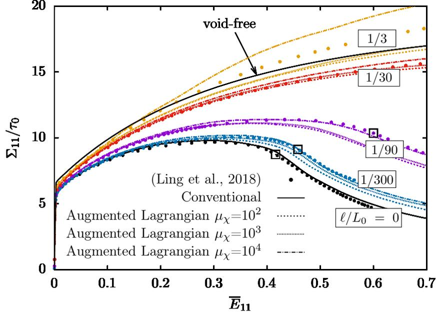
Fig. 15: Macroscopic stress-strain behaviour for different intrinsic length to cell size ratios  $\ell/L_0$  obtained with the micromorphic formulation (dots) by Ling et al. (2018) and the augmented Lagrangian formulation (dashed lines) in porous unit-cell simulations with  $f_0 = 0.01$  and material parameters presented in Table 5. Hollow squares denote onsets of void coalescence.
