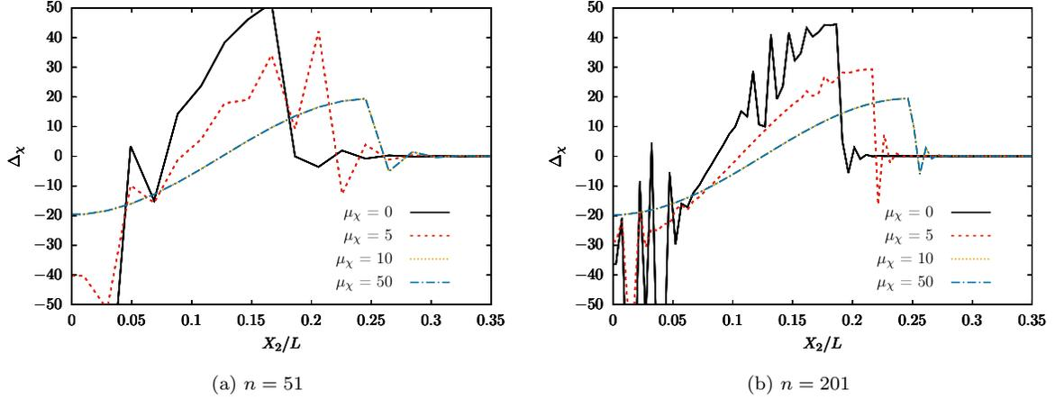
Fig. 2: Numerical solutions of the Laplacian term  $\Delta_\chi$  profile along a periodic strip in simple shear for several values of  $\mu_\chi$ . The discretization is  $n = 51$  elements in (a) and  $n = 201$  elements in (b).
