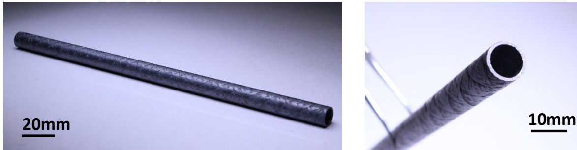
Fig. 2. SiC/SiC composites cladding as processed.
