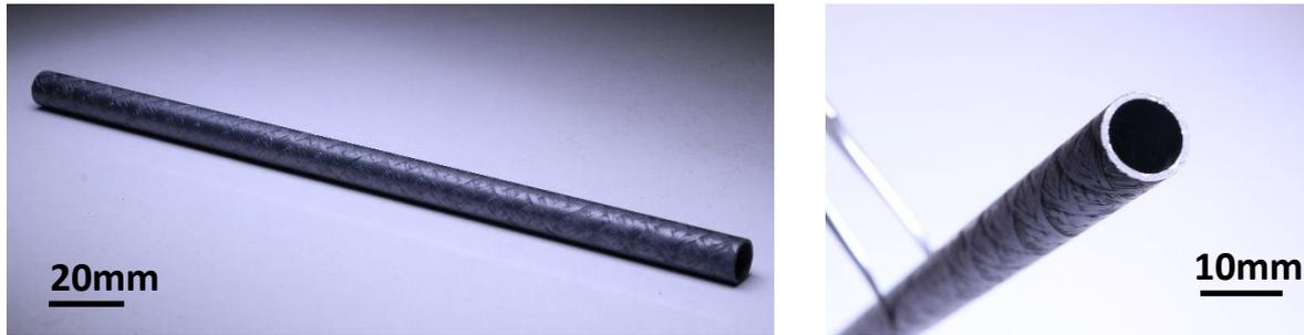
**Fig. 2.** SiC/SiC composites cladding as processed.
