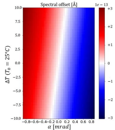
Figure 3: 2D map of the computed angular offset versus  $\Delta\theta_1^\alpha$  and  $\Delta\theta_3^T$  variations
