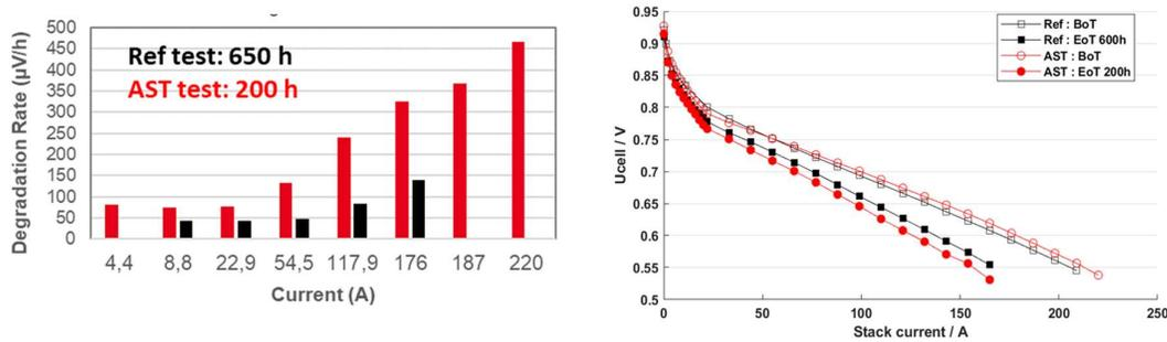
**Figure 2.** ID-FAST average stack cells degradation rates assessed during ageing (left side) and polarization curves (right side) recorded at beginning of test (BoT) and end of test (EoT) for ageing tests conducted under ID-FAST reference dynamic load cycles (in black) or exacerbated load cycles load cycles (in red).
