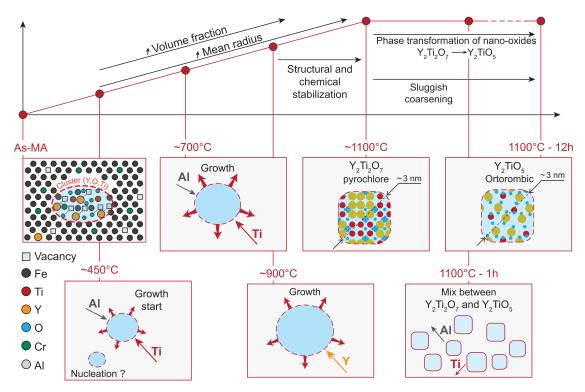
Fig. 14. Scheme outlining the major chemical and structural evolution of the nano-oxides identified throughout the thermal treatment of ODS steels fabrication process.
