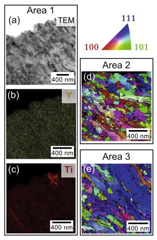
**Fig. 1.** TEM image in bright field (a), with the corresponding TEM/EDS images showing the Y (b), and Ti elemental maps (c) displaying homogeneous distribution of Y and a local Ti enrichment, along with ASTAR orientation mapping showing a highly deformed matrix (d, e) in two different areas of the CP-14Cr specimen.
