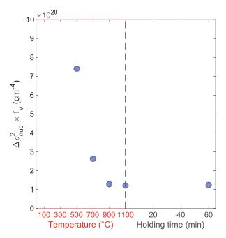
**Fig. 8.** Evolution of the SANS  $\Delta \rho_{nuc}^2 \times f_{\nu}$  on CP-14Cr specimens.
