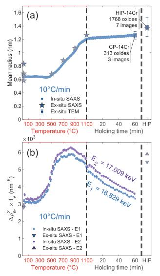
**Fig. 2.** Evolution of the mean radius (a), and  $\Delta \rho_{e^-}^2 \times f_{\nu}$  (b), of the nano-oxides upon a 10 °C/min heating rate on the CP-14Cr and HIP-14Cr specimens extracted from SAXS data.
