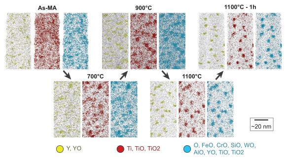
Fig. 10. About 10 nm thick slices of APT 3D reconstructions of the CP-14Cr specimen at different stages of the thermal treatment, from as-MA to 1100 °C - 1 h.
