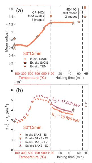
**Fig. 3.** Evolution of the mean radius (a), and  $\Delta \rho_e^2 \times f_v$  (b), of the nano-oxides upon a 30 °C/min heating rate on the CP-14Cr and HE-14Cr specimens extracted from SAXS data.
