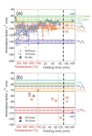
**Fig. 6.** Evolution of the anomalous factor at the Y K-edge acquired at the ESRF synchrotron (a) and at the Ti K-edge acquire at the PSI synchrotron (b), on CP-14Cr, HE-14Cr and HIP-14Cr specimens.
