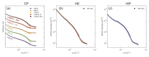
**Fig. 4.** SAXS scattering intensity curves on CP-14Cr specimens, showing the evolution of the precipitate contribution toward lower q-values (i.e. bigger precipitates) (a), HE-14Cr specimen (b) and HIP-14Cr specimen (c), displayed at 4.766 keV along with the fitted model in continuous line.
