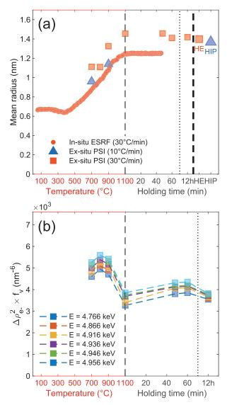
**Fig. 5.** Mean radius evolution at different stages of the interrupted thermal treatment measured at PSI synchrotron and compared with *in-situ* measurements acquired at the ESRF synchrotron (a), and evolution of the  $\Delta \rho_{e^-}^2 \times f_{\nu}$  of the nano-oxides SAXS contributions at several energies close to the Ti K-edge (b), on CP-14Cr specimens.
