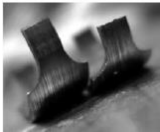
Figure 24: Pictures of fractured specimens after ring tensile testing at room temperature; irradiated Zirlo™ containing ~320 wppm hydrogen after Type B treatment at 350 °C and different effective stresses. Nominal dimensions of the ring are given in [1].
