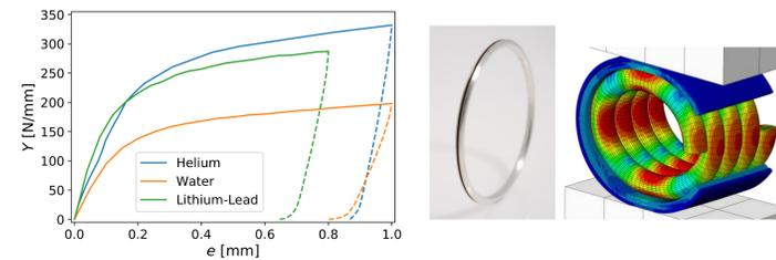
Fig. 3: Load-compression curve of the different seals
