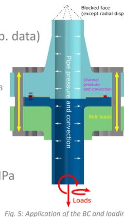
Fig. 5: Application of the BC and loadings
