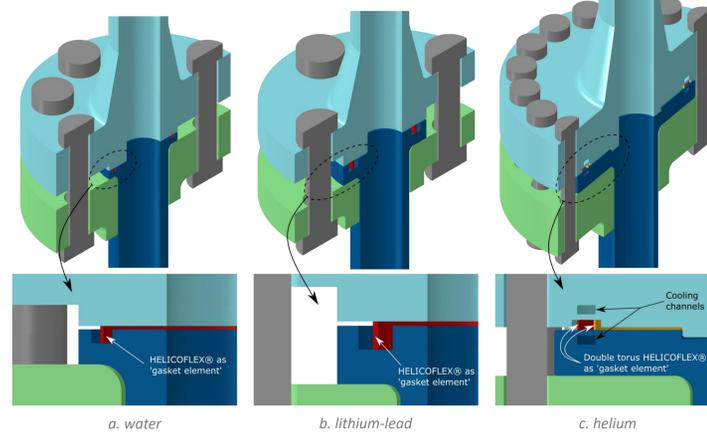
Fig. 2: Simplified half view of the flanges
