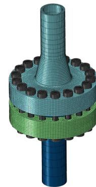
Fig. 4: Mesh of the helium pipe
