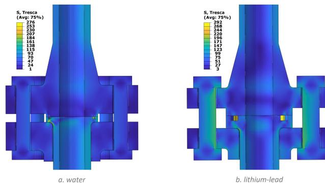
Fig. 6: Tresca equivalent stress (in MPa) in the flanges
