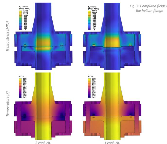
Fig. 7: Computed fields in the helium flange
