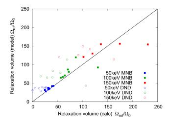
FIG. 9. A comparison of the relaxation volume computed using a full relaxation of the cascade (x-axis) to the relaxation volume predicted using the tabulated fits to the data (Tables III, V, and VII). The diagonal line indicates a 1:1 match i.e., a perfect reproduction of the relaxation volume.
