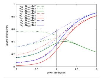
**FIG. 11.** Relaxation volume coefficients for cascades characterized by powerlaws for the size-frequency distributions of interstitial loops and vacancy clusters, with power-law indices  $s_l$  and  $s_V$ . The relaxation volumes per point defect for a cascade can be written as  $\Omega_{rel}/\Omega_0/N_{FP} = 1 + b_0^{(l)} w_{l,0} + b_1^{(l)} w_{l,1} + b_0^{(V)} w_V$ . Vertical lines indicate the power indices measured using MD for 150 keV PKA cascades in tungsten.<sup>85</sup>
