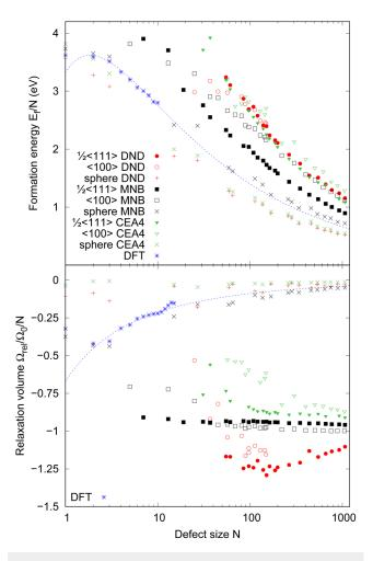
**FIG. 6.** Formation energy and relaxation volumes of low-energy vacancy defect clusters. The loops were generated with circular shapes, and the voids as spheres. DFT computed energies of the low-energy vacancy clusters from Ref. 46, with an extrapolated line fitted to  $E_f = a_0 N^{2/3} + a_1$ . DFT computed relaxation volumes for the same structures in Ref. 46 fitted to  $\Omega_{rel}/\Omega_0 = b_0 N^{2/3} + b_1$ .
