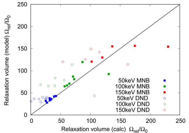
**FIG. 9.** A comparison of the relaxation volume computed using a full relaxation of the cascade (x-axis) to the relaxation volume predicted using the tabulated fits to the data (Tables III, V, and VII). The diagonal line indicates a 1:1 match—i.e., a perfect reproduction of the relaxation volume.
