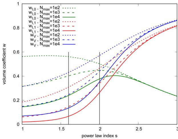
**FIG. 11.** Relaxation volume coefficients for cascades characterized by power-laws for the size-frequency distributions of interstitial loops and vacancy clusters, with power-law indices  $s_I$  and  $s_V$ . The relaxation volumes per point defect for a cascade can be written as  $\Omega_{rel}/\Omega_0/N_{FP} = 1 + b_0^{(I)}w_{I,0} + b_1^{(I)}w_{I,1} + b_0^{(V)}w_V$ . Vertical lines indicate the power indices measured using MD for 150 keV PKA cascades in tungsten.<sup>85</sup>
