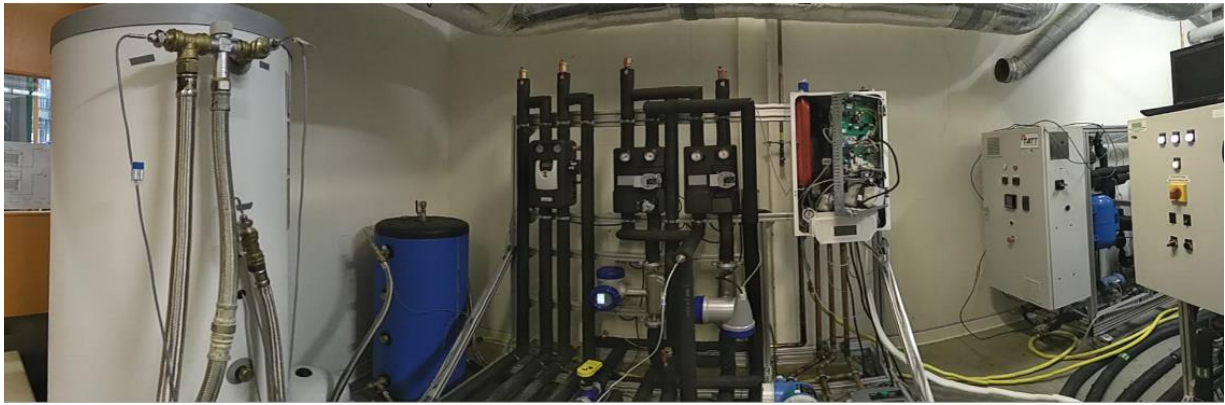
Fig. 3: HS1 concept and outlook of real prototype integrated in semi-virtual test bench
