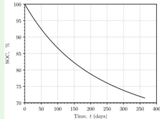
Thermodynamics and kinetics make the electrolyte density, cell voltage, and SOC decrease exponentially, showing that the lower the SOC, the lower the selfdischarge phenomenon.
