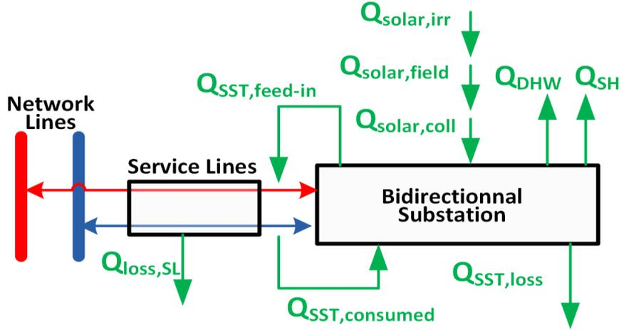
Fig. 6: Schematic representation and nomenclature associated to thermal power fluxes (Q) around the substation
