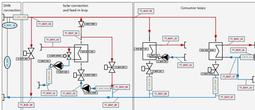
Fig. 1: Technical drawing of the BSST prototype
