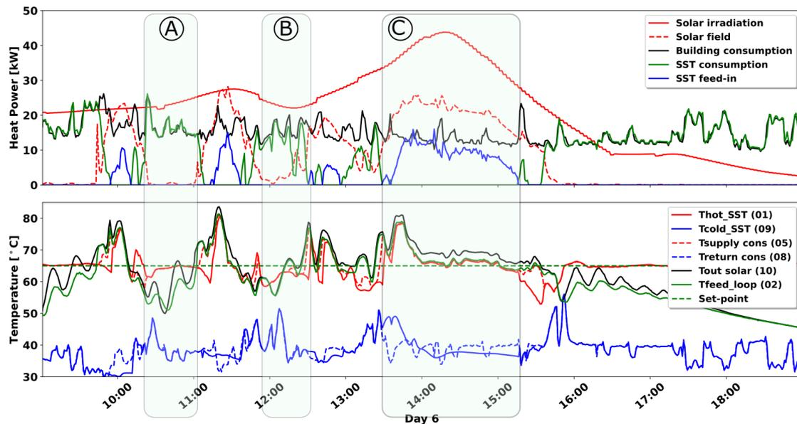
Fig. 7: Experimental results obtained for day 6 of the sequence (Top: heat power; Bottom: Temperatures)
