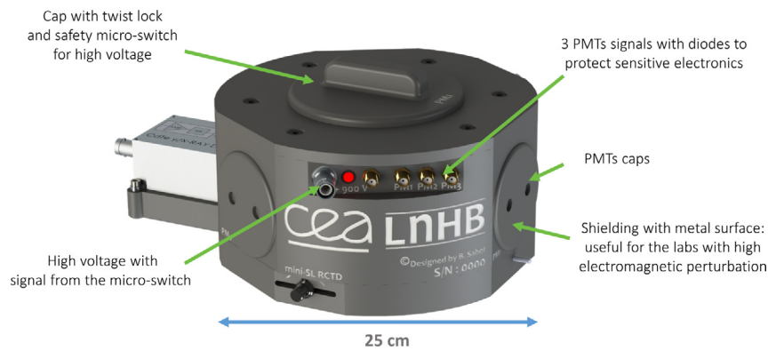
Fig. 1. 3D illustration of the mini-TDCR device. Its large size is due to additional components that can be included in the system: an external photon-emitting source with a collimator and a gamma detector (NaI(Tl) or Ce(Br) 0.5 inch size and CdTe). With these components the system can be used as a Compton spectrometer.
