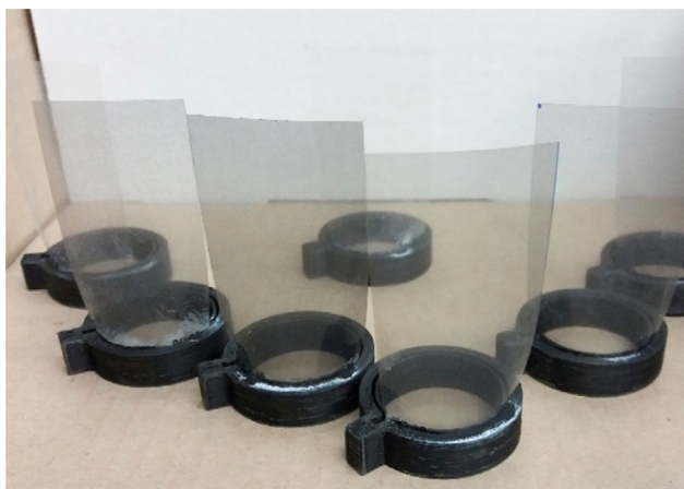
Fig. 9. Filters with different neutral density. The filters shown here were designed to cover only one PMT.
