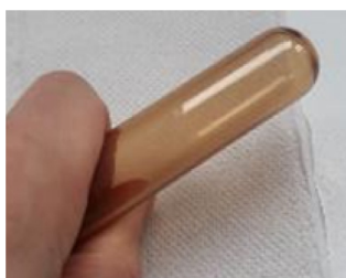
Fig. 11. Picture of the irradiated glass; the brown colour is due to a defect of the glass after exposure to Co-60 gamma rays.
