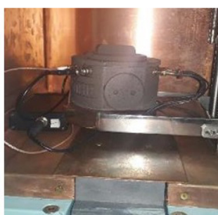
Fig. 18. Picture of the micro-TDCR device inside the shielding from an HPGe detector.
