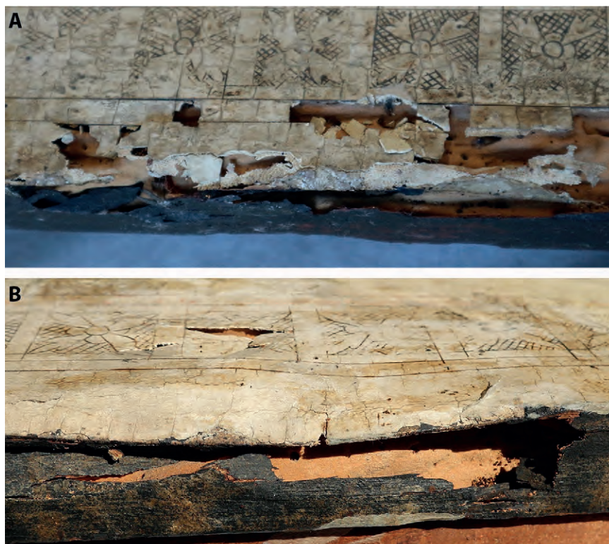
Figure 5 | Details of some deep insect galleries in the cross (© E. Rabelo/ V. Demonty).
