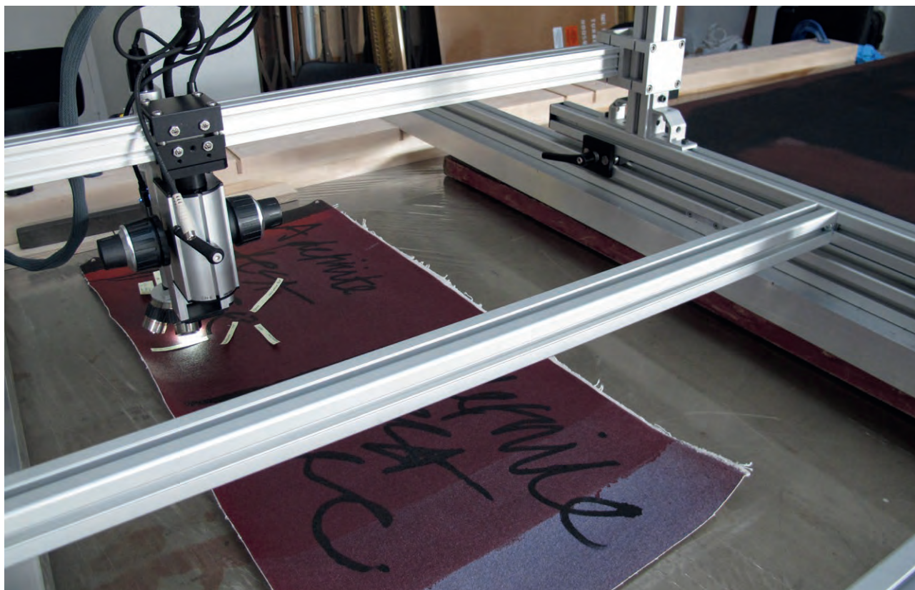
Figure 4 | A portion of the aged and tagged representative sample under the Hirox digital microscope during the testing phase. Photo Bronwyn Ormsby © Tate.
