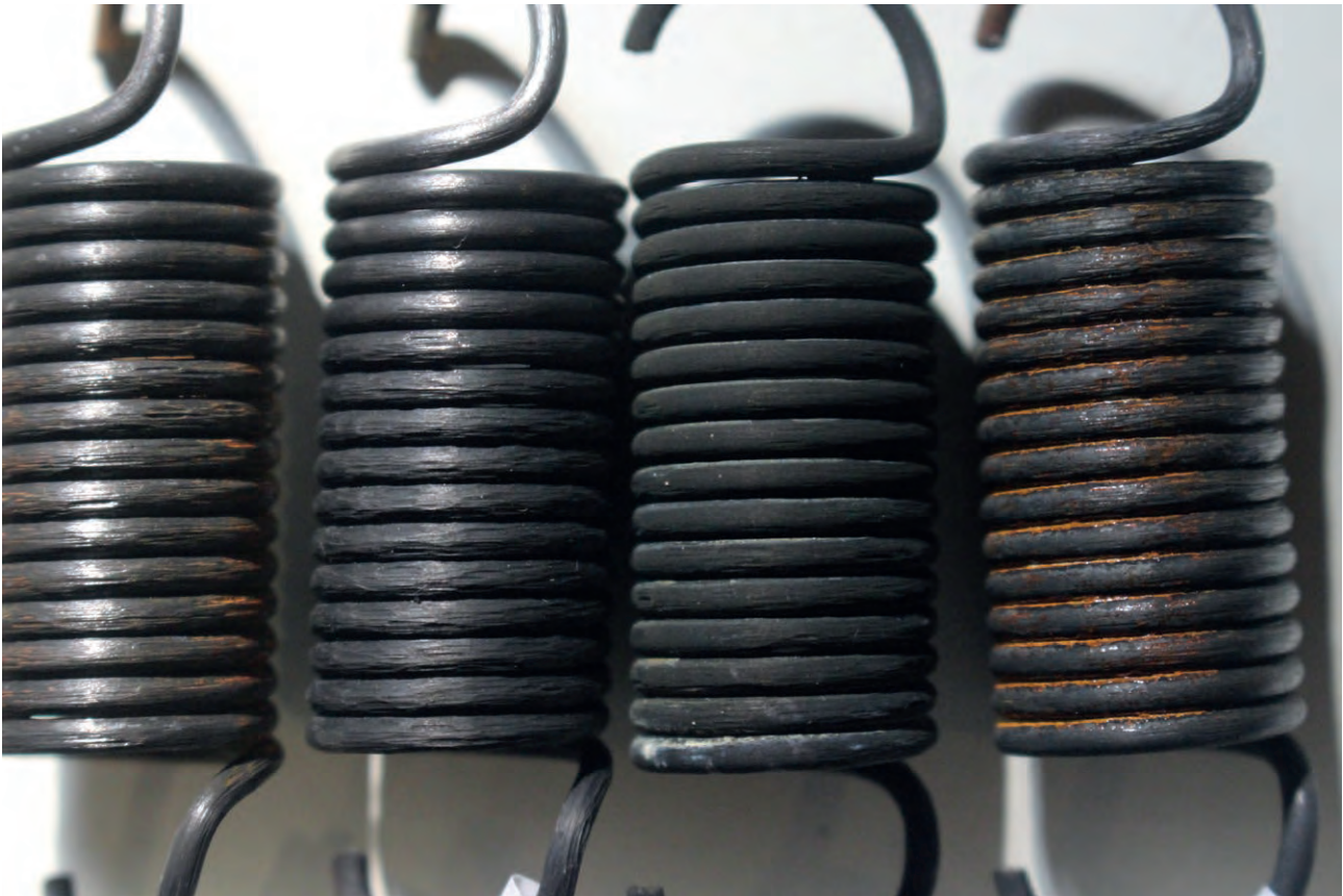
Figure 5 | Low-carbon steel wire mock-ups showing the results of various submersion tests performed. The second from the left represents the executed treatment. Photo by the author ©.
