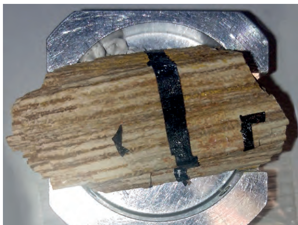
Figure 5 | Fossil sample (length 41.64 mm) from the petrified forest at Ban Tak, Thailand on SEM-EDS sample holder. The carbon tape circumferencing the sample is a non-destructive alternative to coating. Smaller pieces are used as indicators of points of interest.
