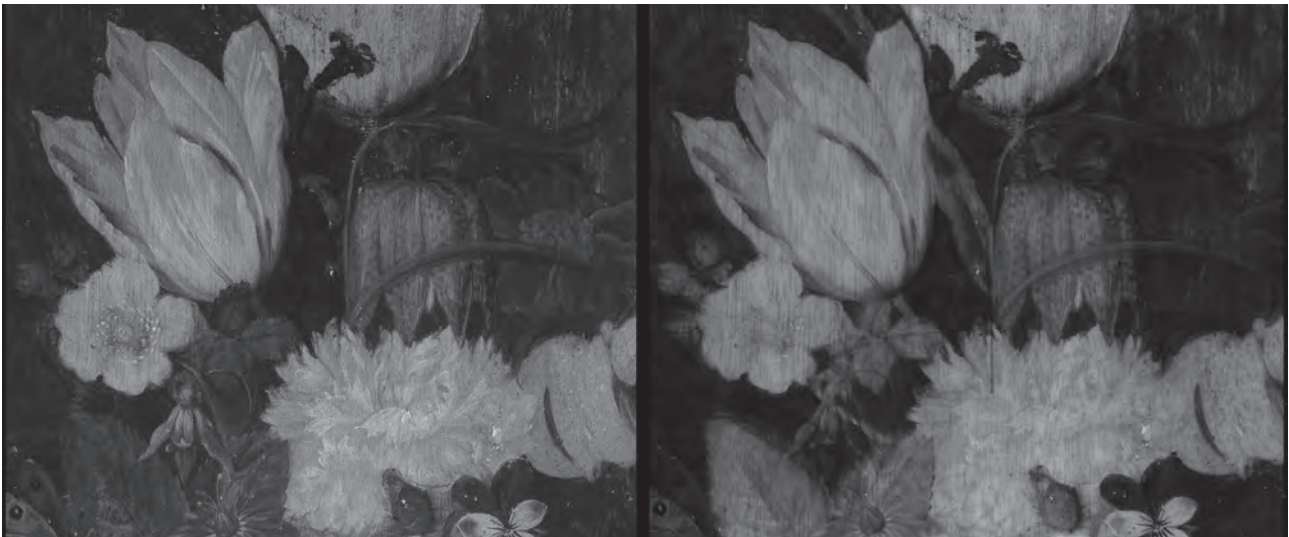
Figure 6 | Reflected infrared detail taken with a modified Lumix camera (IR range 850-1000 nm) showing the opacity of the hyacinth blossoms at shorter wavelengths (left); Reflected infrared detail taken with an Osiris infrared camera (IR range 900-1700 nm), showing the transparency of the blossoms at longer wavelengths (right).
