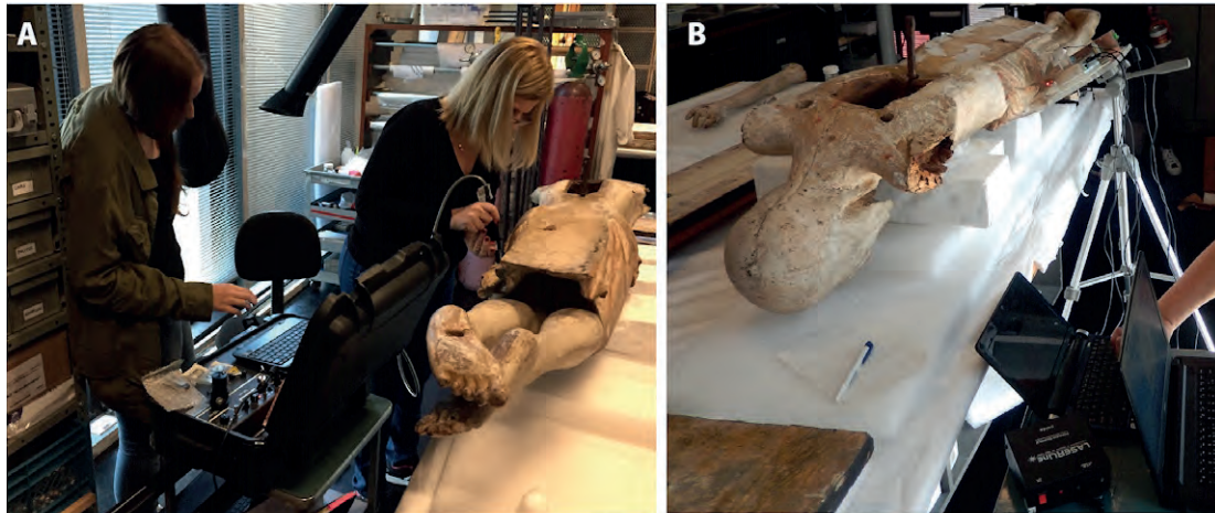
Figure 4 | Analyses being performed: A. Raman spectrometry; B. XRF (© E. Rabelo/ V. Demonty).
