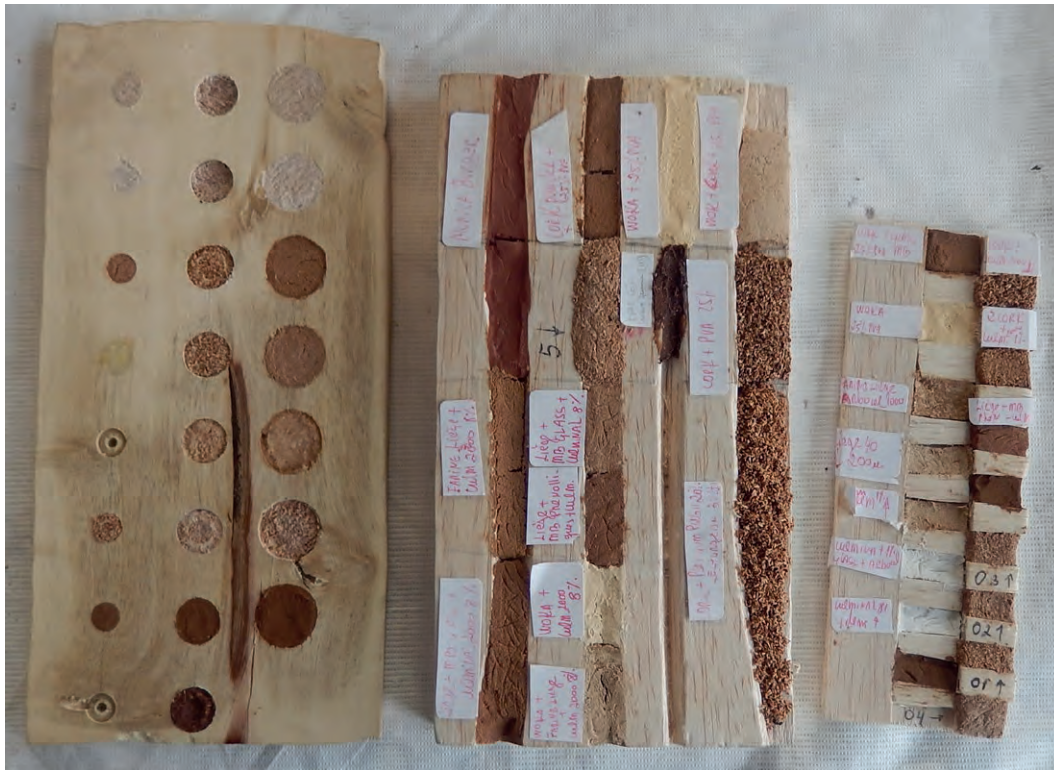
Figure 6 | Filling tests completed before the treatment. (© E. Rabelo/ V. Demonty).
