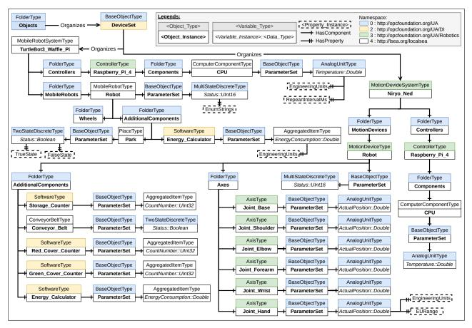
Fig. 3. Excerpt of the blueprint of the OPC UA information system for the PAL monitoring case study
