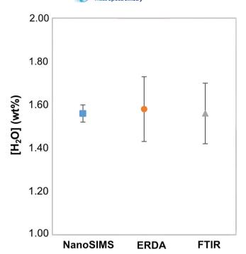
**FIGURE 4** Comparison of water concentrations in staurolite obtained by the three methods FTIR, ERDA and NanoSIMS. Results are similar with 1.56 ( $\pm$  0.14), 1.58 ( $\pm$  0.15), and 1.56 ( $\pm$  0.04) wt% H<sub>2</sub>O, respectively [Color figure can be viewed at wileyonlinelibrary.com]
